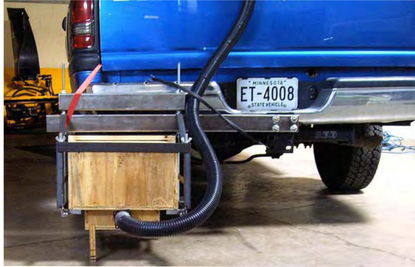
This mobile dust collector, based on a device designed by Ado and Sanders called the Colorado State Dustometer, was built by the research staff.
