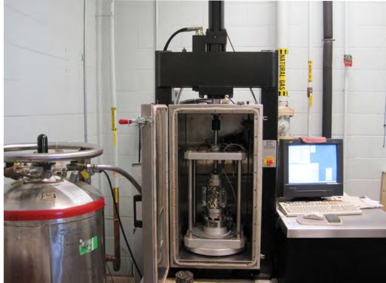
Dynamic modulus tests were used to evaluate various RAP mixtures over a range of temperatures.
