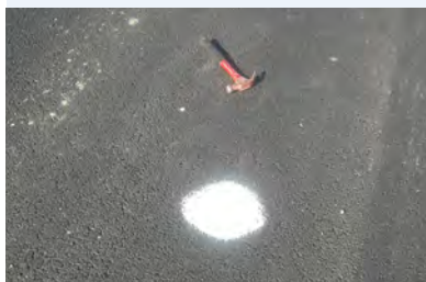
Sand patch testing involves spreading a set volume of sand to measure surface texture.
