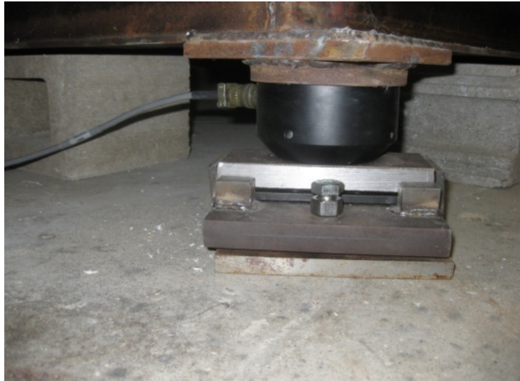
Figure C-3: Load cell installed under device
