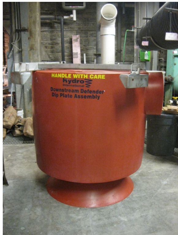
Figure A-18: Photo of the Downstream Defender insert used at SAFL
