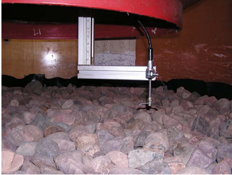
Figure 5-6: ADV positioned above the river rock bed
