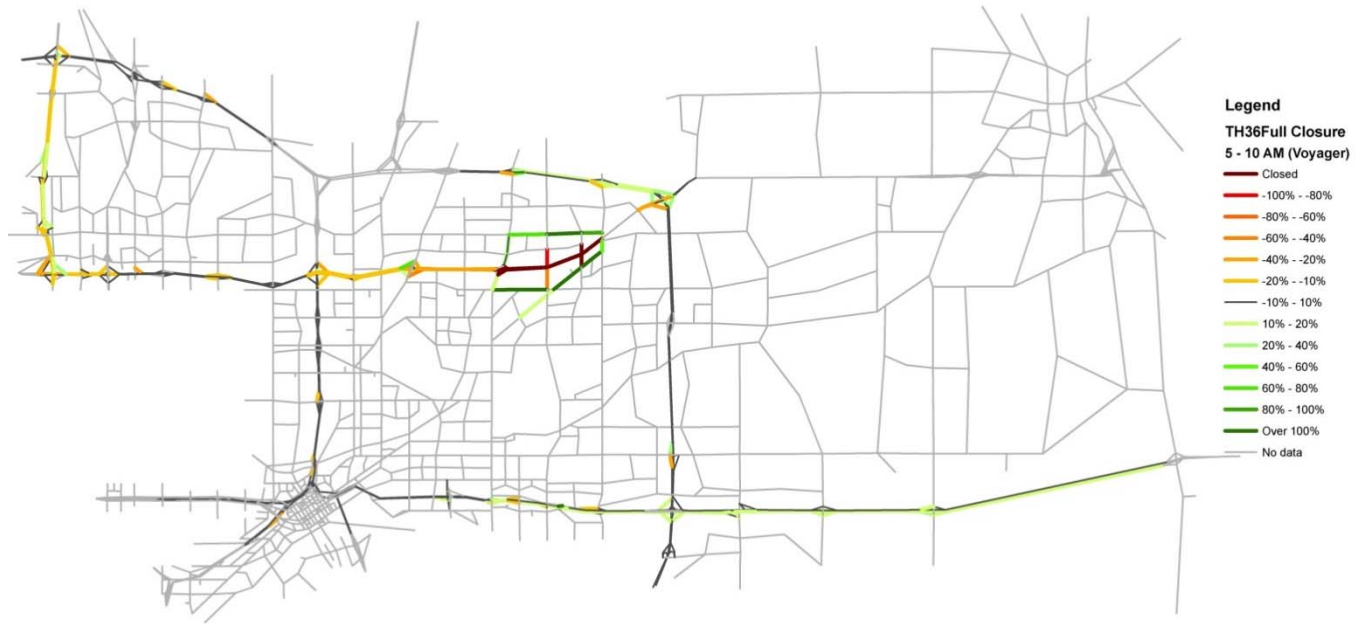
Figure 52 Traffic diversions in AM (real data)
