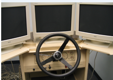
The STISIM simulator uses three PCs to generate a virtual environment presented on 17-inch monitors.
