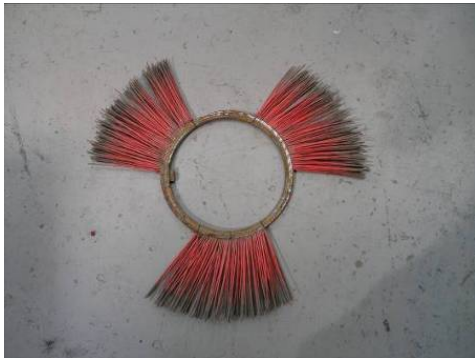
Brush and spring tine components for the reel
