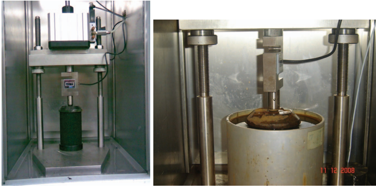
Figure 3-2. Flow number test setup
