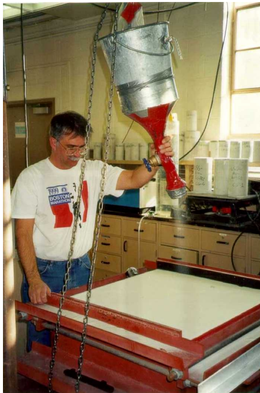
Figure 5. Cubical Test Bin, Sand Raining Operation.
