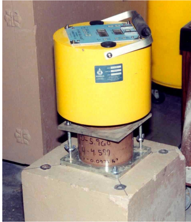
Figure 16. GeoGauge Test on Soil on Concrete Pedestal (note acrylic mold).
