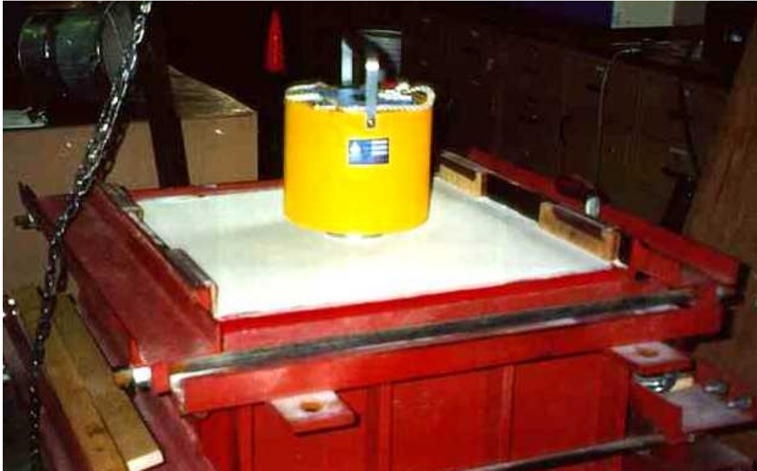
Figure 6. Cubical Test Bin, Stiffness Evaluation by GeoGauge.
