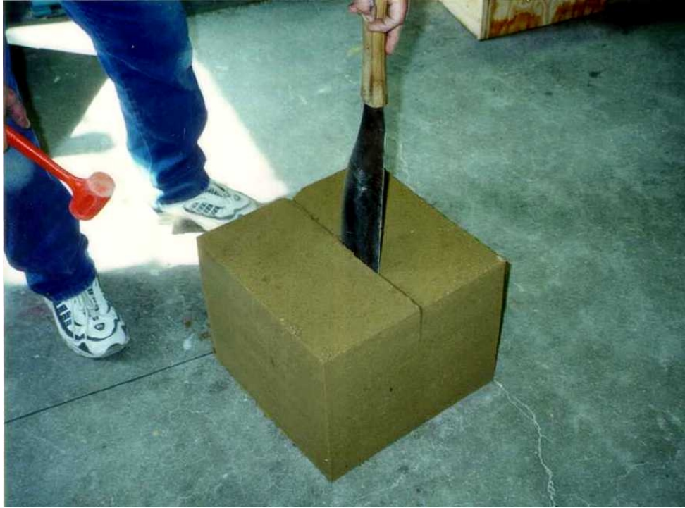
Figure 14. Moisture Content Evaluation (Full Depth).
