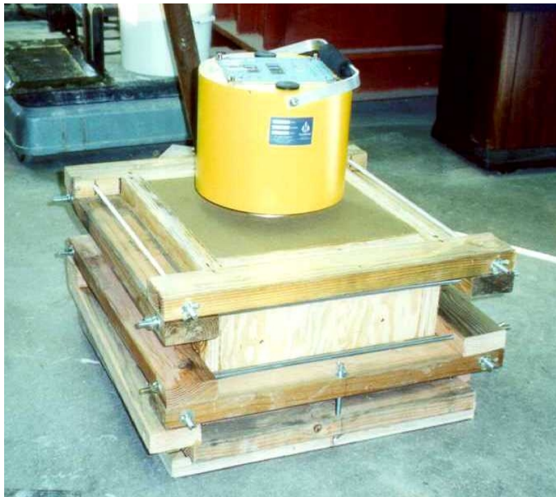
Figure 13. GeoGauge Testing on Plywood Soil Bin with Cohesive Soil.
