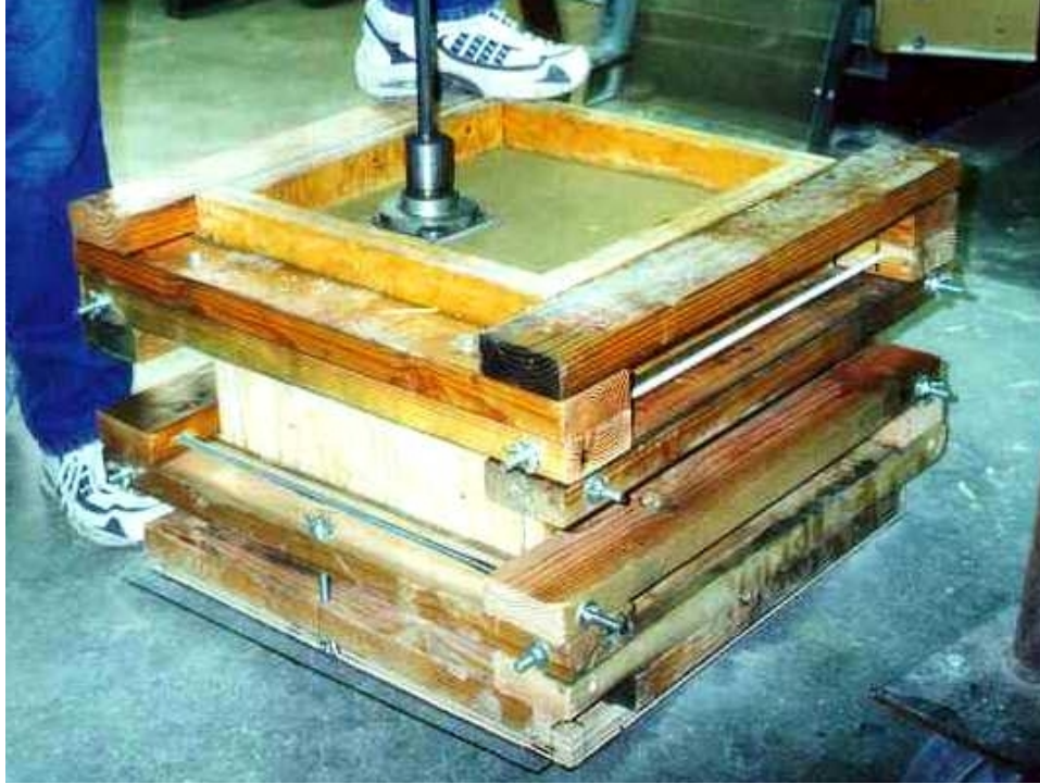
Figure 12. Plywood Soil Bin for Cohesive Soil (note compaction hammer).
