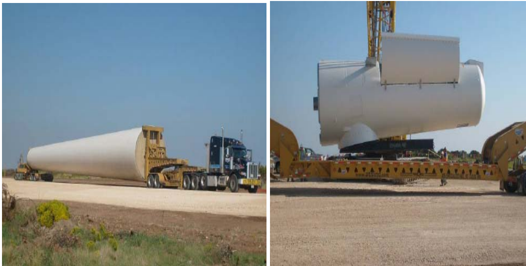
Figure B1. Shipping of Wind Turbine.
