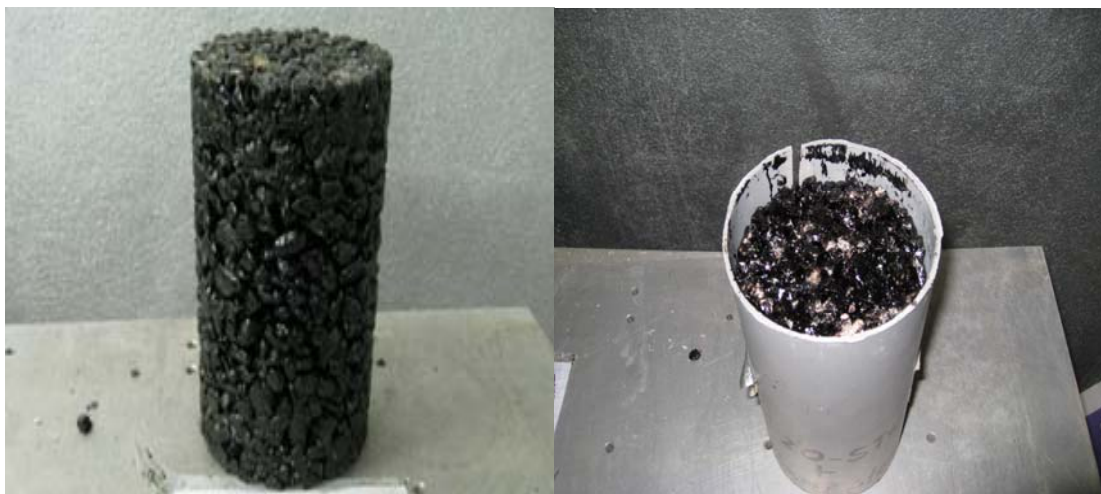
Figure 16. Molded Seal Coat Mixture.
