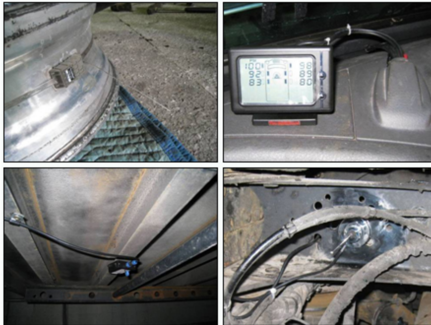
Figure 10. Grouped photo. HCI Tire-SafeGuard components.
