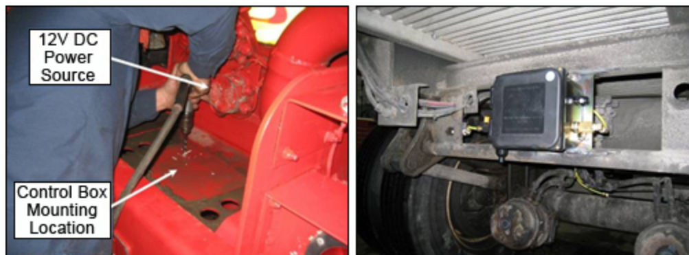
Figure 18. Grouped photo. CLI and GFS control box installation between taillights (right) and on tanker's crossbeam (left).
