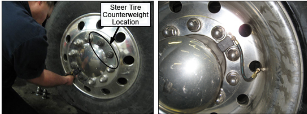
Figure 8. Grouped photo. Module installation of steer wheel (left) and drive wheel (right) with steer tire counterweight location.
