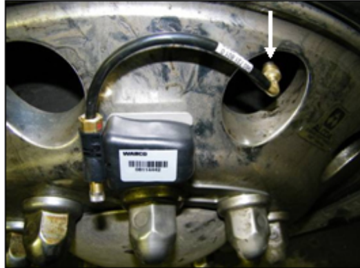
Figure 29. Photo. IVTM wheel module installation.
