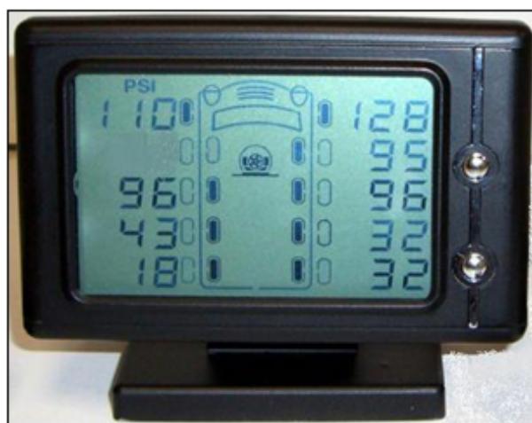
Figure 40. Photo. Tire-SafeGuard reliability; display missing left inside tire data (GFS).
