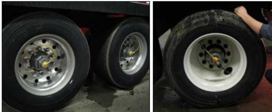
Figure 16. Grouped photo. MTIS, rotary units on wheel ends.
