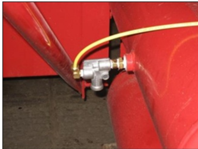
Figure 15. Photo. Pressure protection valve (CLD).
