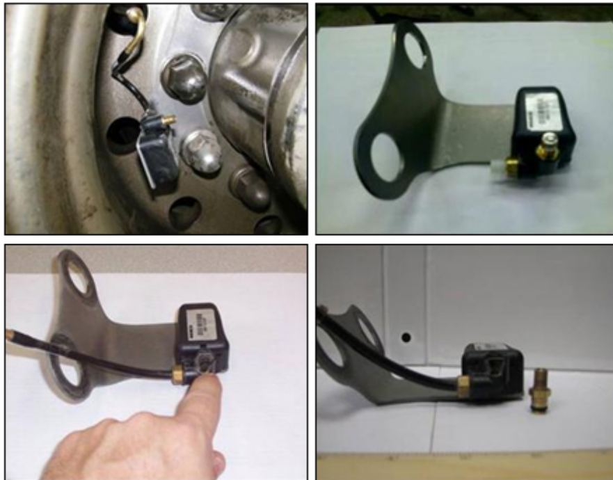
Figure 28. Grouped photo. Second-generation wheel module (fill valve) failure.
