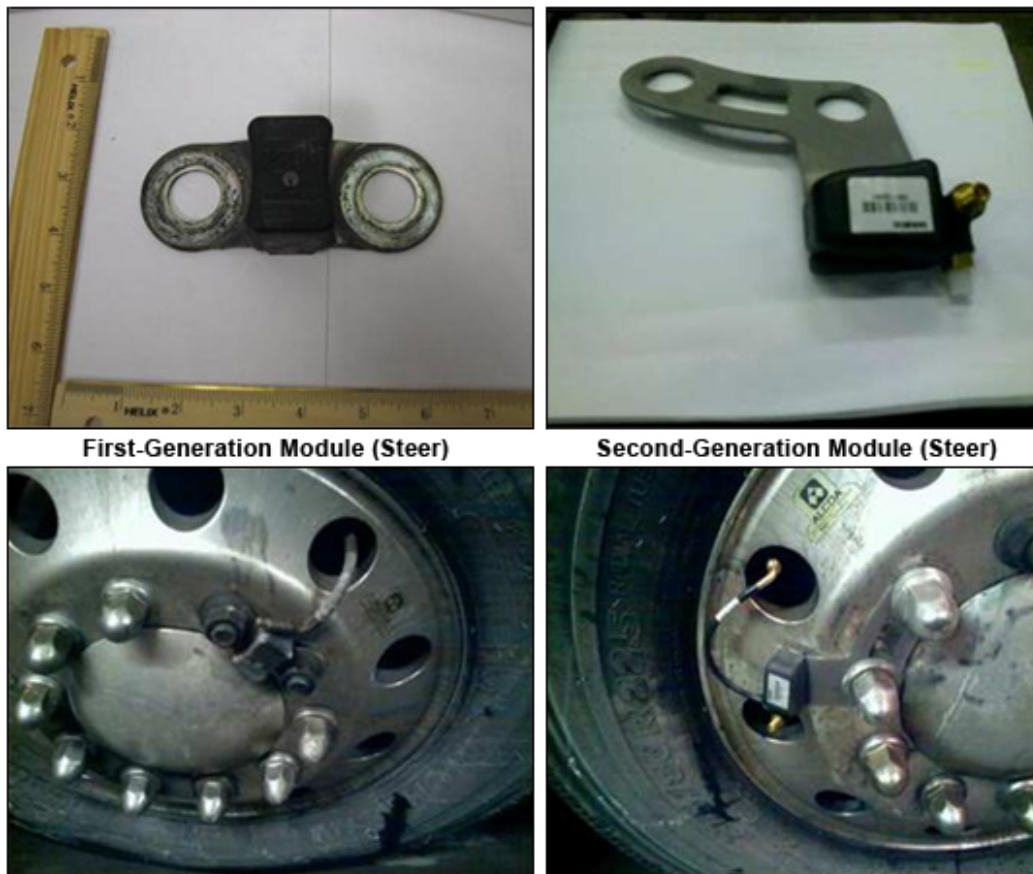
Figure 27. Grouped photo. Wabco wheel modules, side-by-side comparison of first-generation and second-generation modules.
