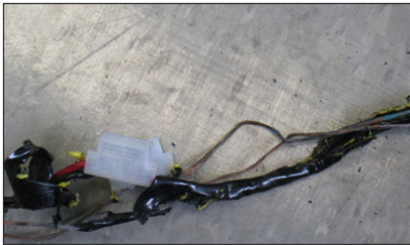
Figure 41. Photo Tire-SafeGuard reliability; failed wire harness.
