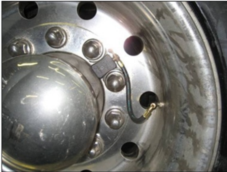
Figure 6. Photo. Wabco IVTM sensor unit mounting system.
