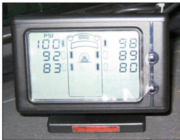
Figure 39. Photo. Tire-SafeGuard reliability, displaying tractor tire data only (GFS).
