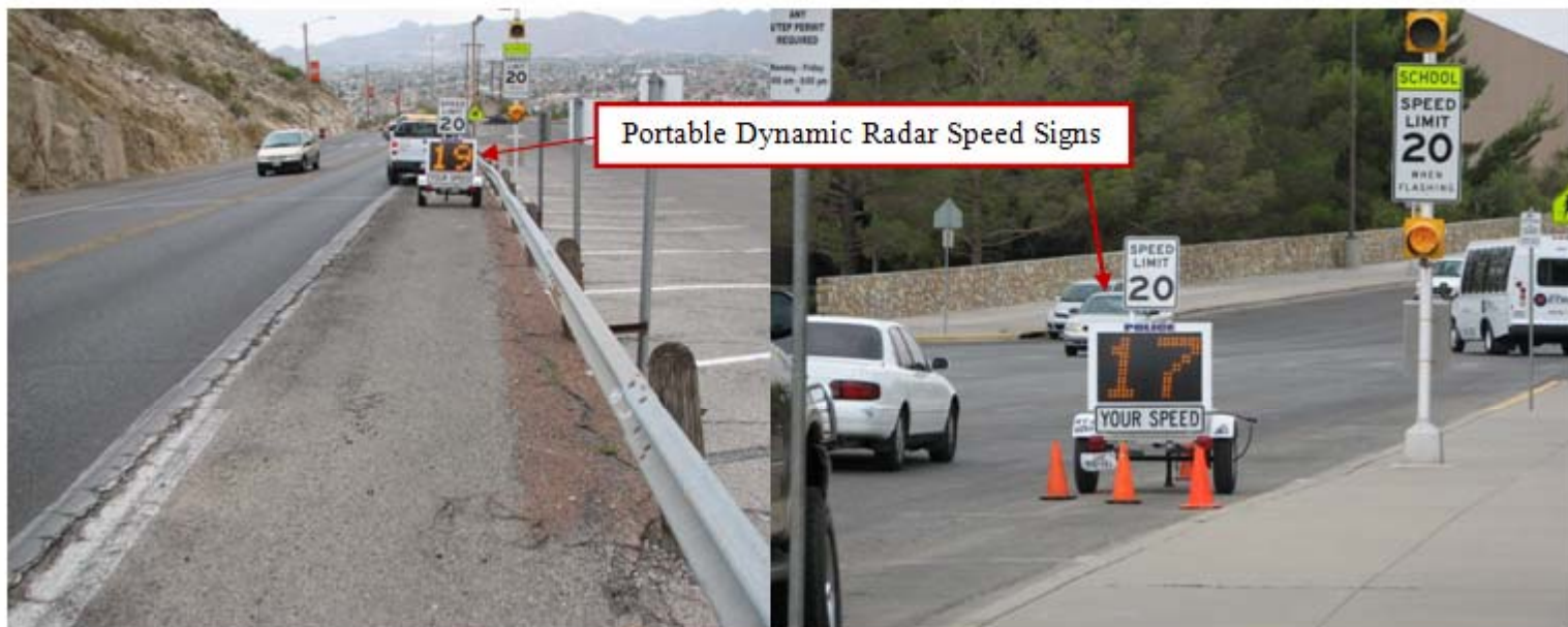
Portable Radar Speed Signs Proved to be Effective in Controlling Traffic along Sun Bowl Dr.
