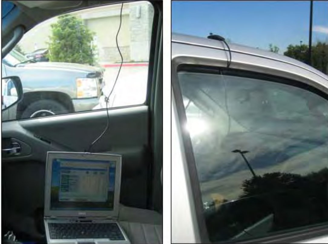
Figure 2. GPS and Software Setup in Vehicle to Record Travel Times
