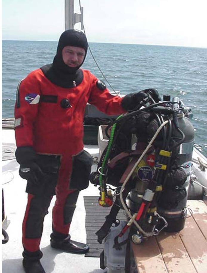
Figure 9. Mr. Eric Takajian (diver) with this diving gear, 2 aluminum tanks and one tank filled with oxygen used for decompression for longer dive.
