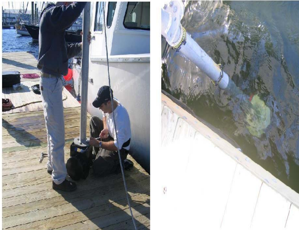
Figure 8: Left panel. The installation of the Farsounder sonar by the Farsounder Inc. engineering crew. Right panel: Sonar in operation.
