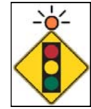
CFSSA located 710 ft before stop bar
