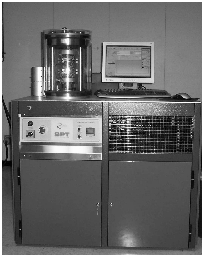
Figure 1. Photograph of the IPC Global Asphalt Mixture Performance Tester.
