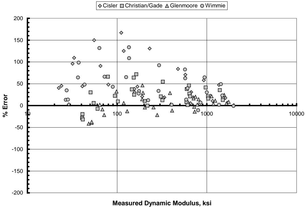
Figure 39. Comparison of Measured and Viscosity Based Witzak Equation Predicted Dynamic Modulus Values.
