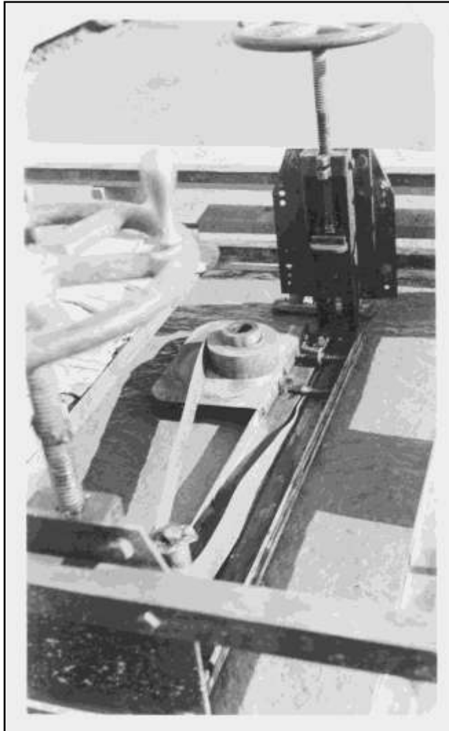
Figure 57 - Continuously fed parting strip
