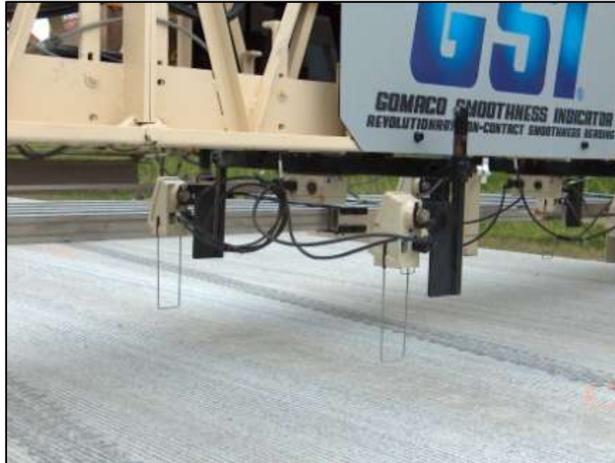
Figure 78 – Noncontact smoothness profile equipment (GOMACO)
