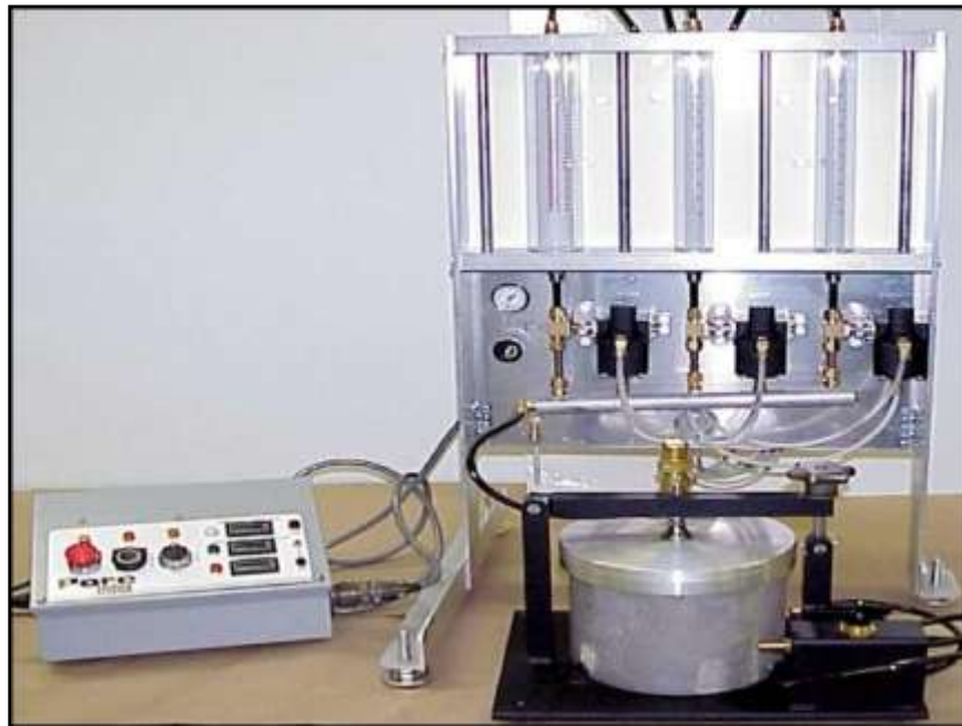
Figure 10 - Iowa Pore Index test equipment
