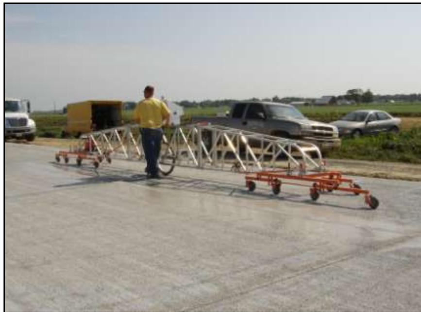
Figure 66 - 25 foot California type profilograph
