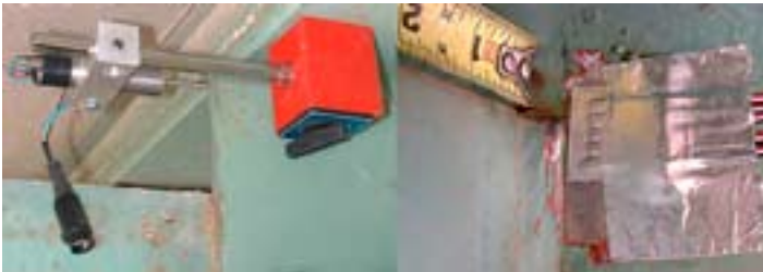
Figure 23 - The out-of-plane behavior of the web in a typical web gap location was determined by using both displacements and gradient-strain gauges.
