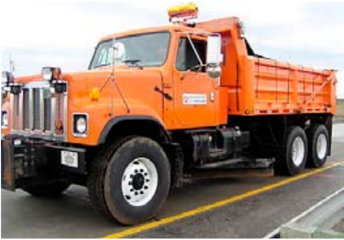
Figure 10 - Iowa DOT tandem-axle load test truck
