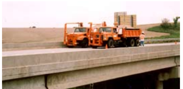
Figure 19 - Load test with two test trucks in adjacent traffic lanes; deflections were measured using displacement transducers on tripods and high-strength wire.
