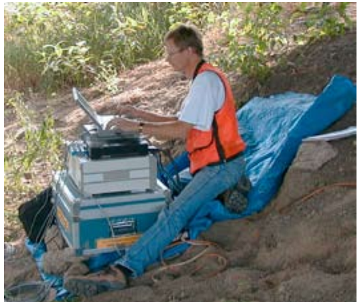
Figure 1 - An instrumentation and data collection system that allows time efficiency and effective monitoring is critical to a load testing program.
