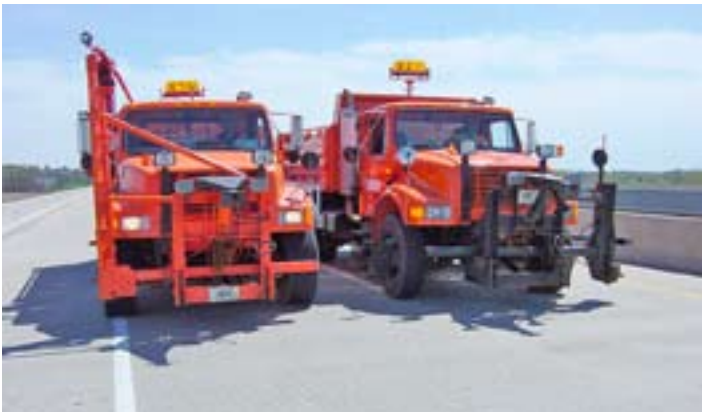
Figure 36 - Test trucks for load rating prior to passage of superload vehicle
