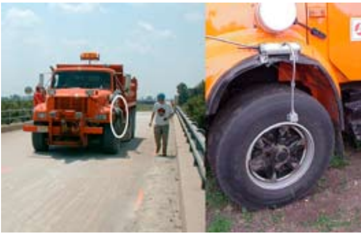
Figure 7 - A test truck crosses the bridge at 5 mph in predesignated driving lanes. To automatically record the truck's position during a load test, hardware devices are mounted to its wheel and fender.
