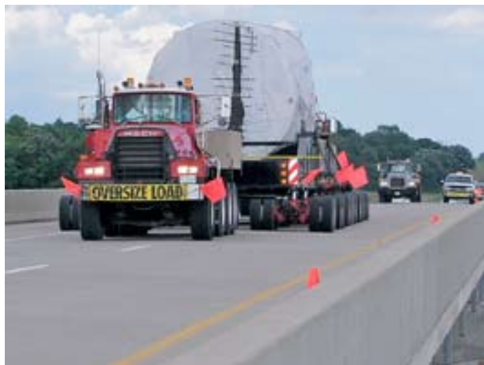
Figure 39 - Superload crosses prestressed girder bridge during load rating test
