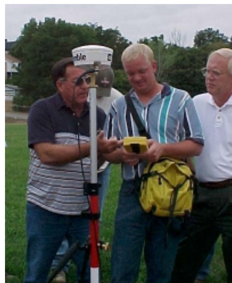
Pat Kliethermes (center) of the Jefferson City Public Works Department demonstrates how to locate a point using the GPS receiver.
