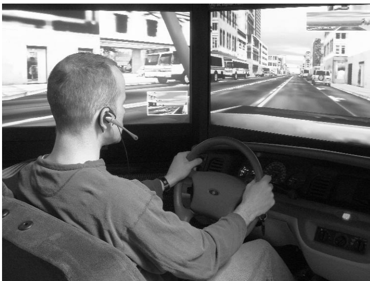
Figure 1. A participant talking on a cell phone while driving in the GE-ISIM driving simulator.
