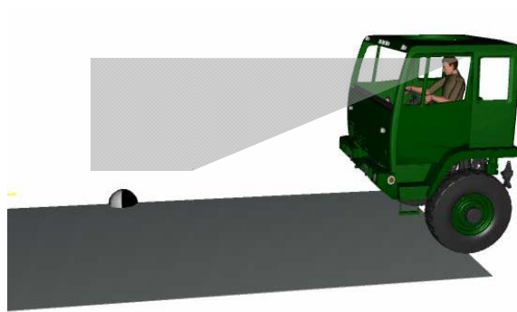
Figure 3. A discrete hazard may pass out of the driver's view at close range due to occlusions caused by the vehicle
