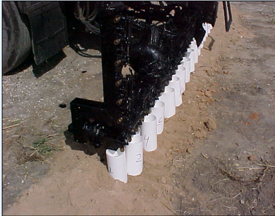
Figure 4 – Cylinders Placed Under the Nozzles
