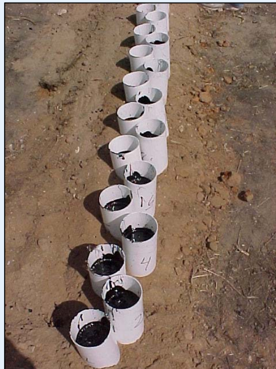
Figure 5 – Cylinders \frac{3}{4} Filled with Asphalt
