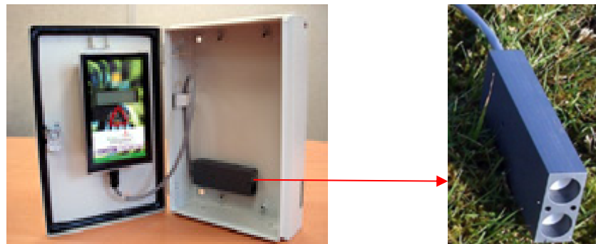
Figure 2. Double pyroelectric sensor by EcoCounter (13)
