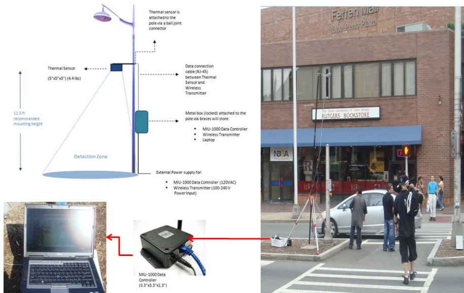
Figure 12. Thermal sensor data extraction
