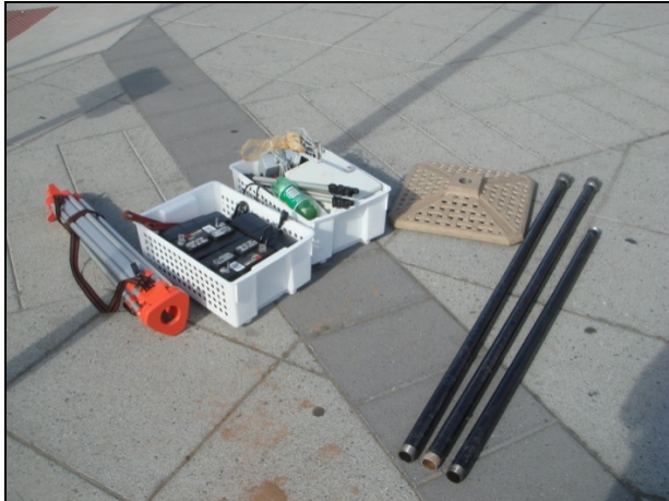
(a) Customized tools for sensor deployment
