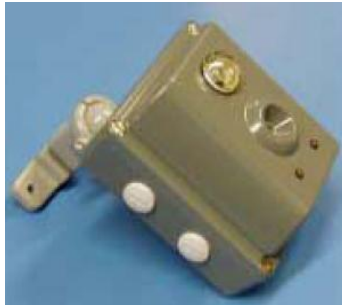
Figure 3. Thermal counter by TrafSys
