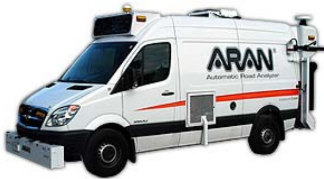
Figure 8: ARAN Automatic Road Analyzer
