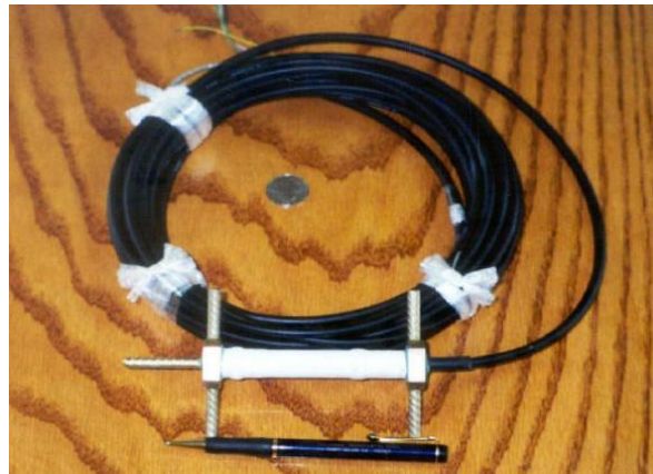
Figure 4 Pressure cells and strain gages used to measure pavement responses
