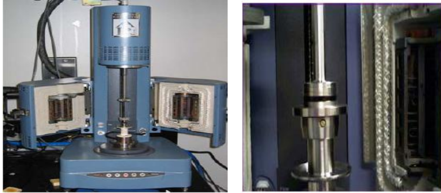
Figure 9 AR 2000 instrument in dynamic shear mode
