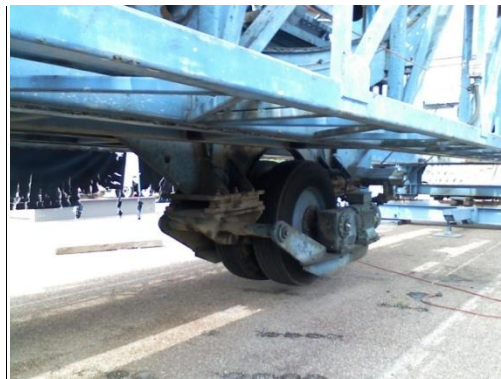
Figure 1 The Louisiana accelerated loading facility
