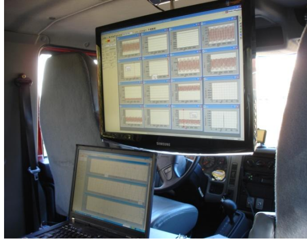
Figure 4.14: Monitoring the LVDTs output signals during loading.
