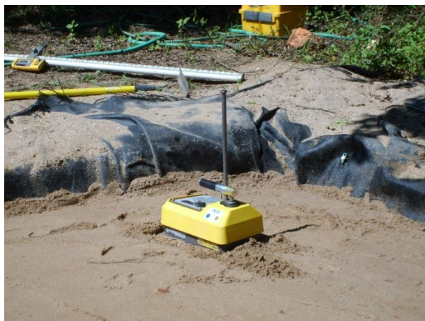
Figure 3.12: Nuclear density gauge reading.
