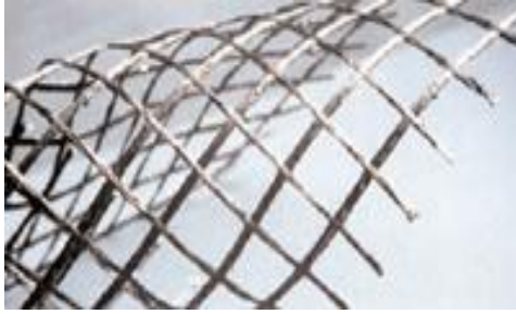
Figure 3.2: Geogrid used in this project (Mirafi® BXG12) ( www.tencate.com ).
