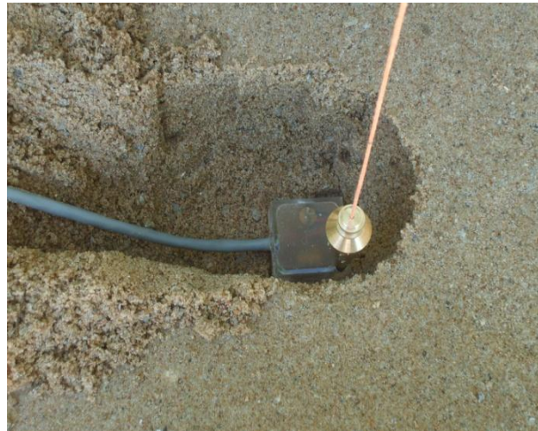
Figure 3.15: Geophone package placement three inches deep in sand lift.
