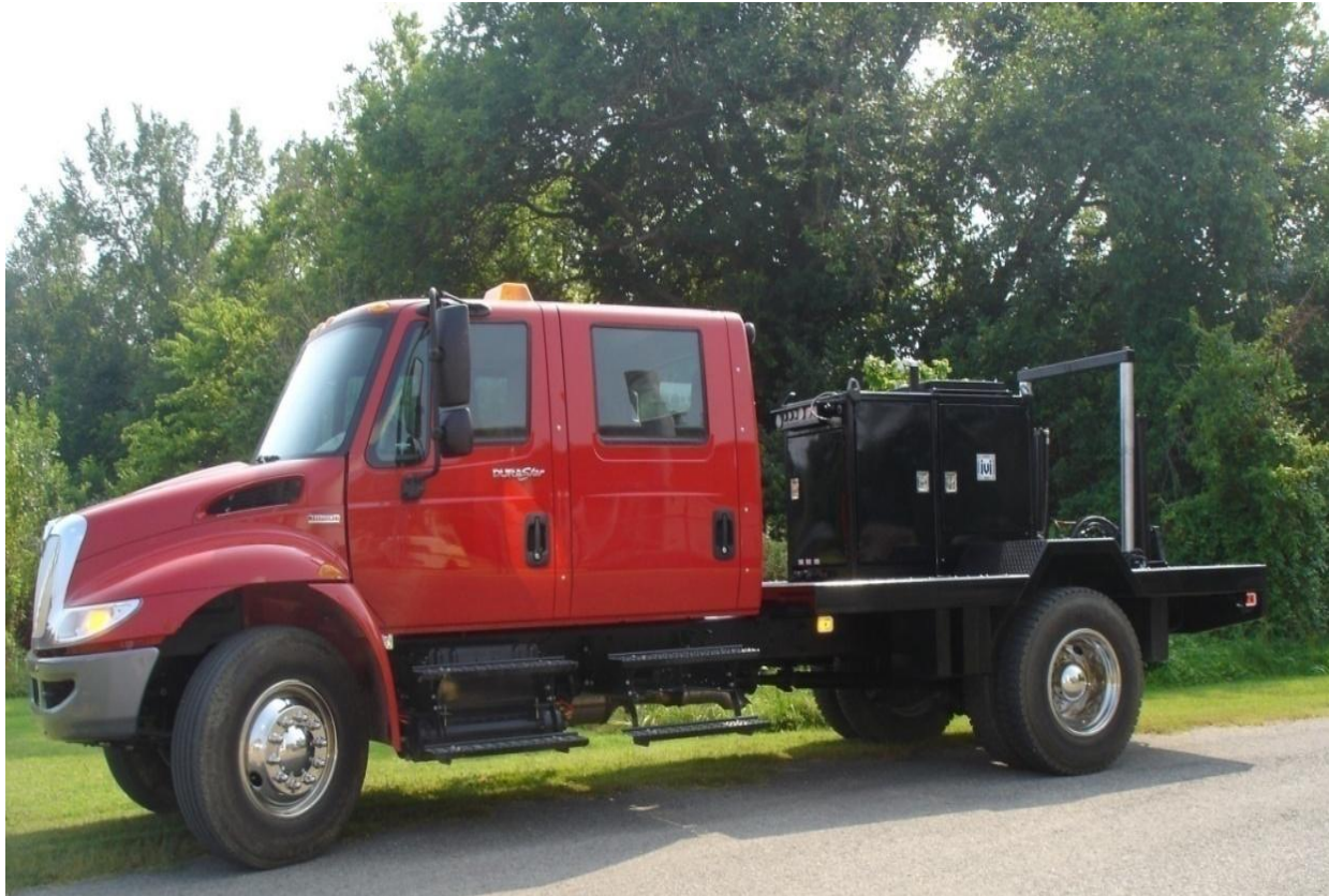
Figure 3.19: University of Arkansas' Vibroseis truck.
