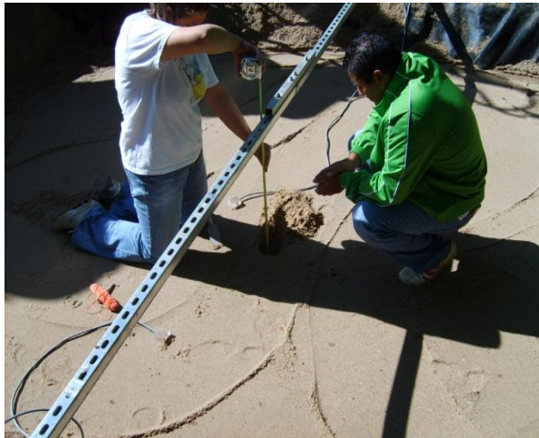
Figure 3.14: Geophone package placement measurements.
