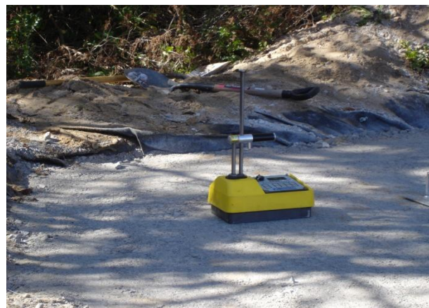
Figure 4.6: Nuclear density reading on the Class 7 base course layer.
