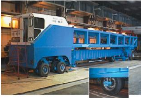
Figure 2.1: Heavy Vehicle Simulator (Perkins et al. 2005).
