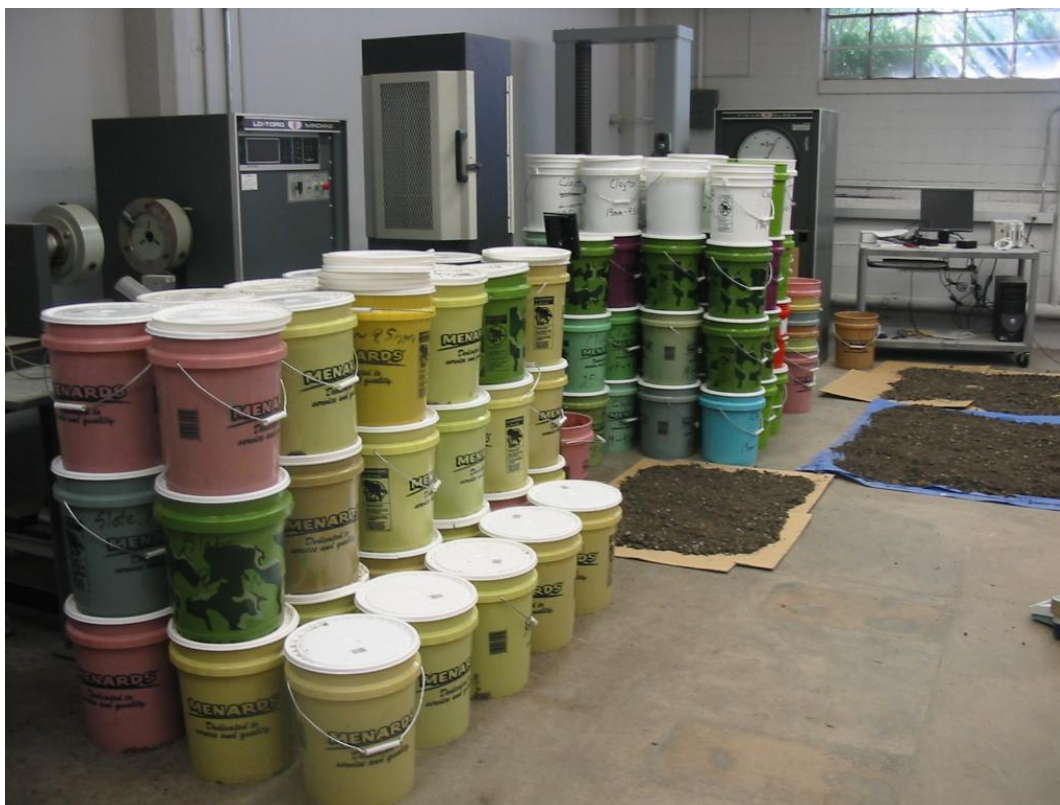
Figure 5-2. Sorted RAP materials in 5-gallon buckets
