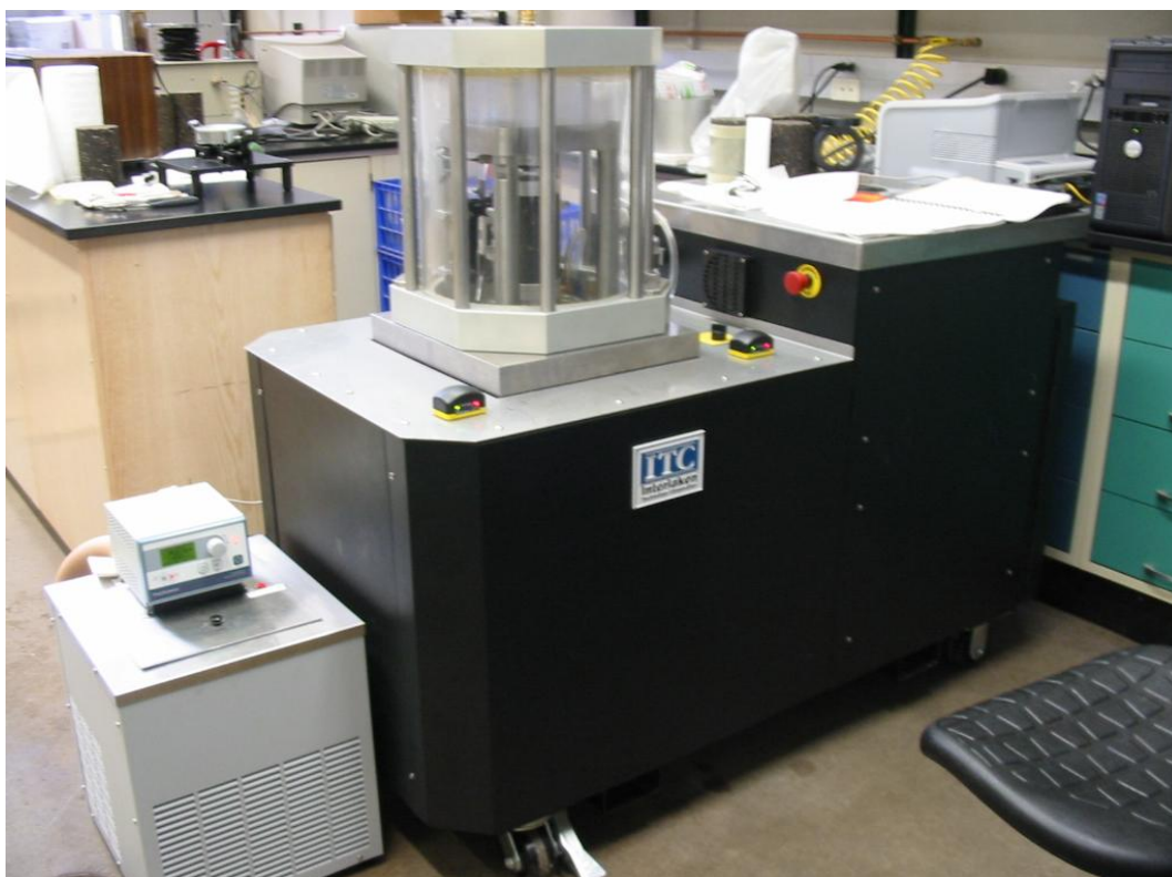
Figure 8-2. Simple performance testing equipment
