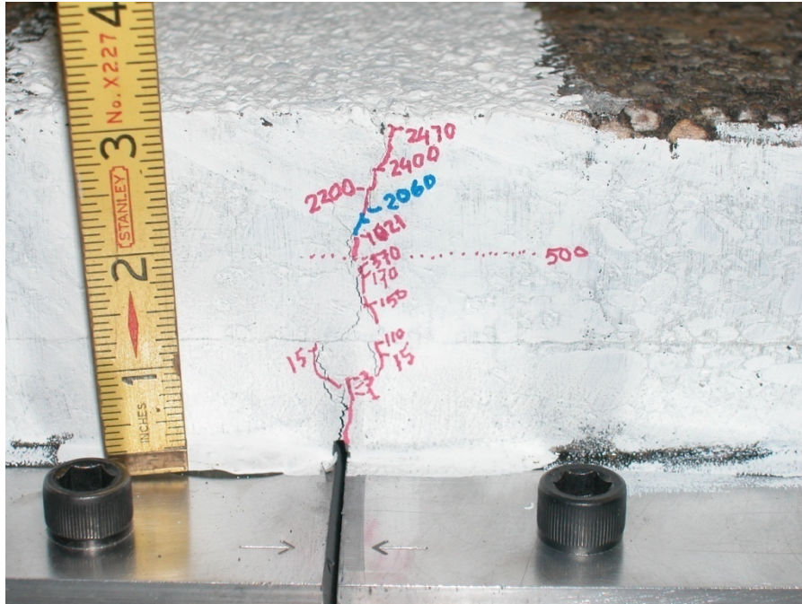
Figure 4-6. Monitoring of Crack Propagation with Large Specimens.
