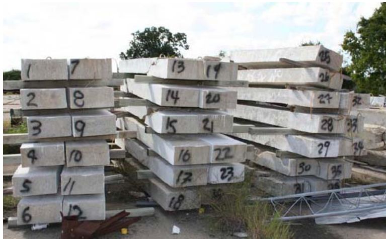
Figure 5-2. Storage Positions of GFRP-Reinforced Beams.
