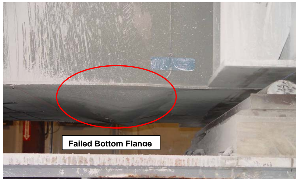
Figure 7.1 Failed Bottom Flange on Hold Down Side
