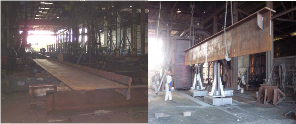
Figure 3.4 SAC Welding of Top Flange/Web and View of Assembly Prior to Shot Blasting
