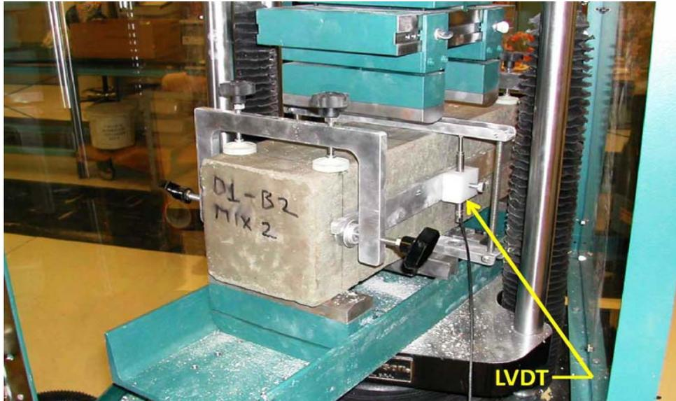
**Figure 6-10. Beam specimen undergoing flexural strength testing.**
