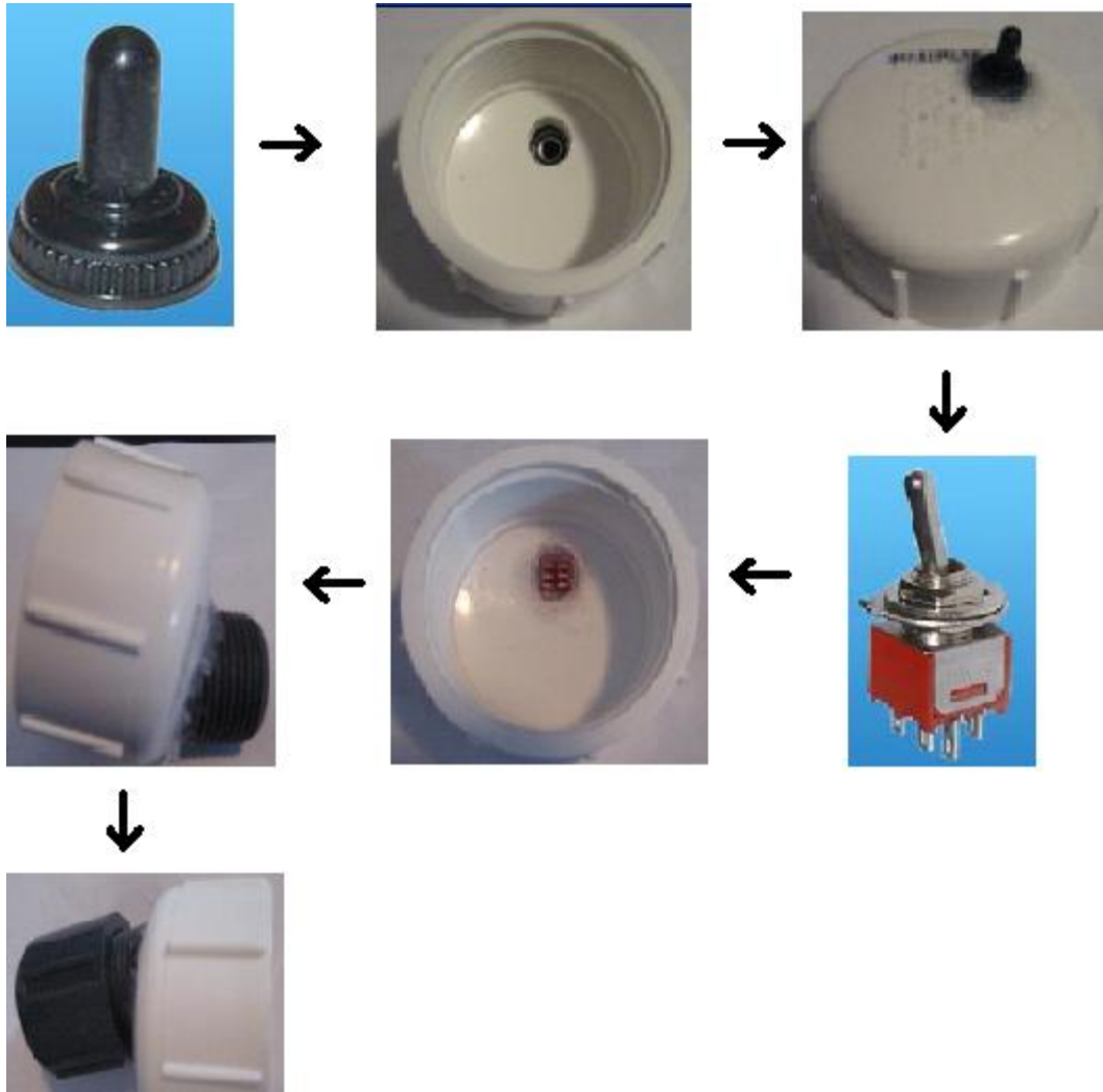
Figure 83: External Arm Switch Construction Steps
