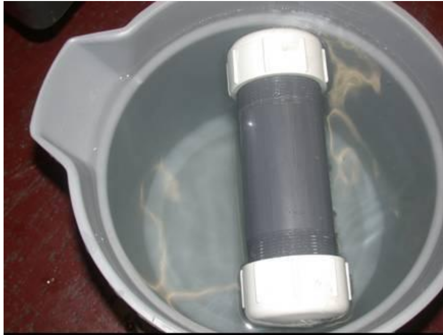
Figure 58: Capsule Floating with No Additional Weight Added
