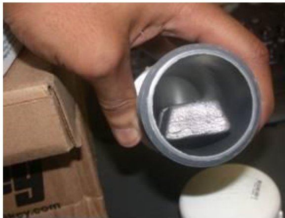
Figure 61: Weight Added to Keep Capsule Submerged for Water Tightness tests.
