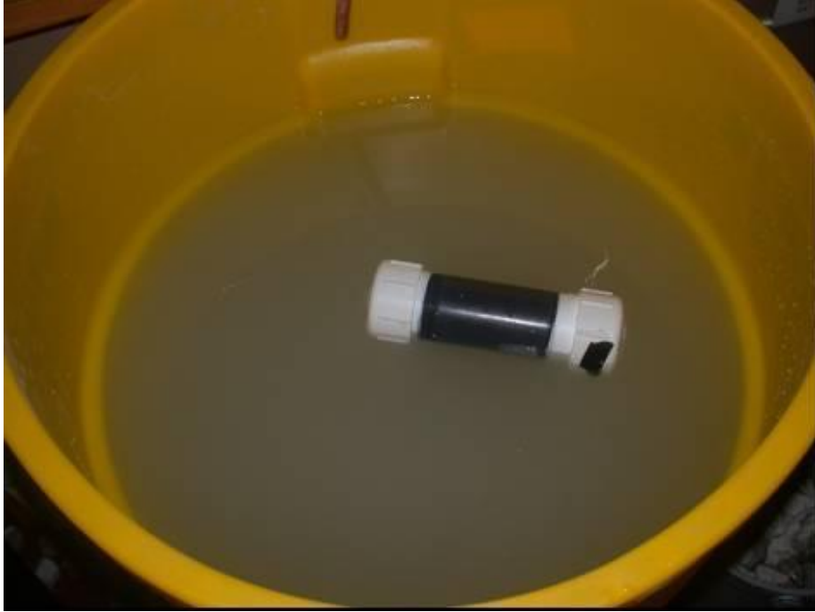
Figure 71: Sensor Unit After Release from Aggregate
