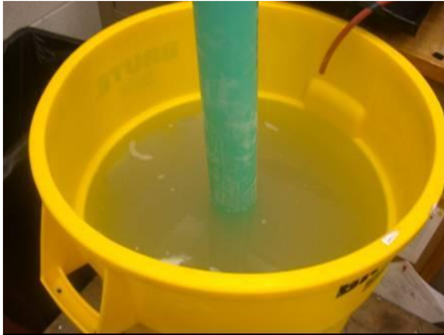
Figure 69: Container with Aggregate, Pipe, and Water
