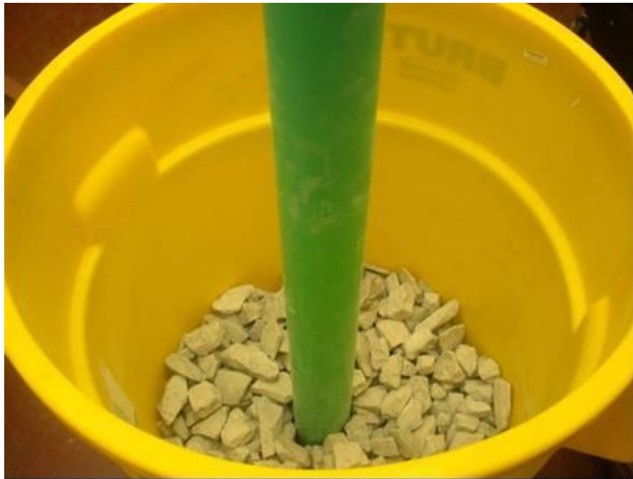
Figure 68: Container with Aggregate and Pipe
