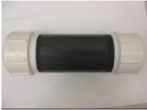
Figure 63: Capsule with Teflon Tape Added.
