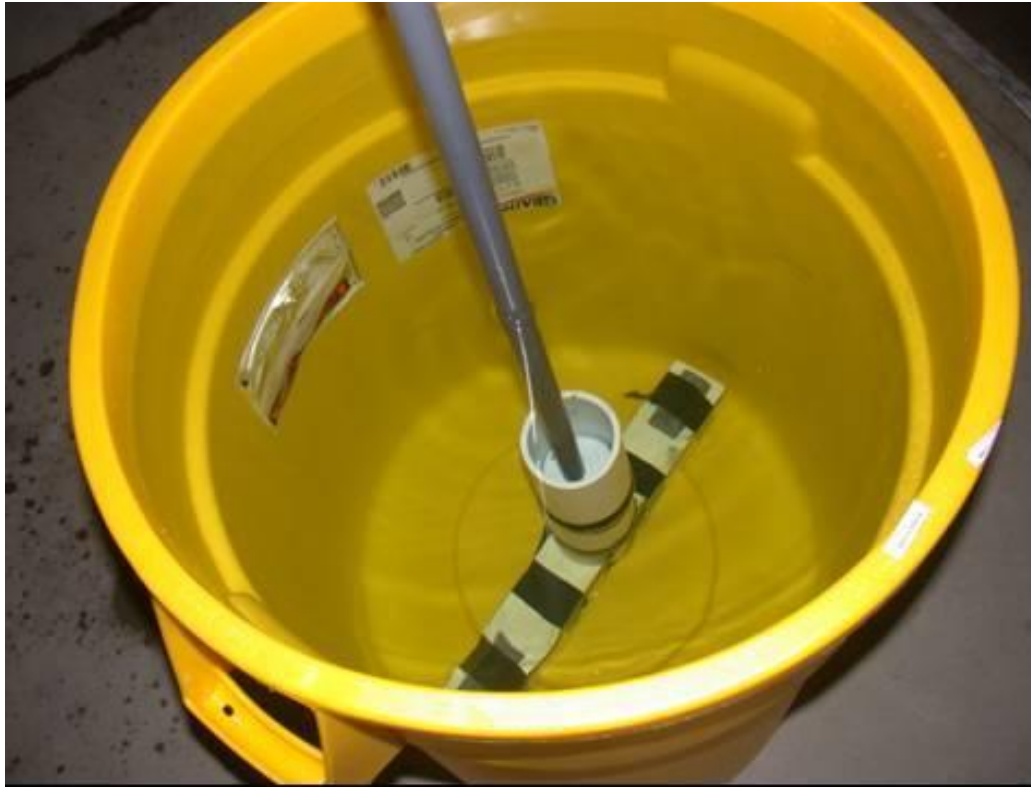
Figure 59: Rise Time Test Before Capsule Release
