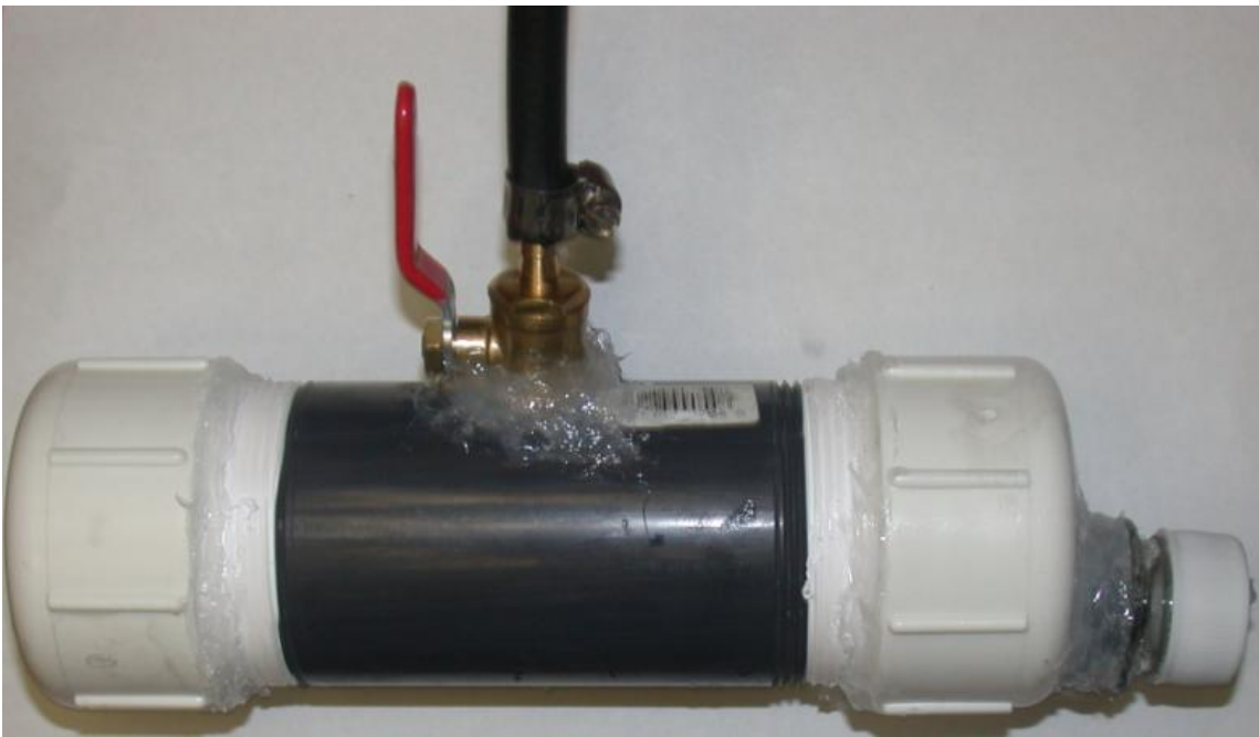
Figure 65: Capsule with Valve and Hose Attachment for Pressure Testing
