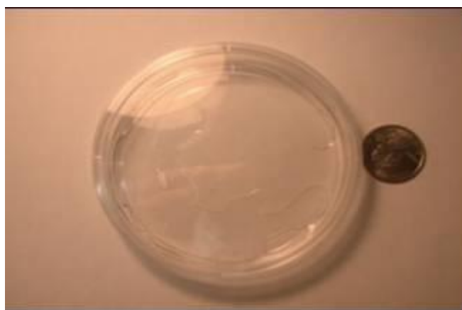
Figure 62: Water Collected from the First Water Tight Test Using Only the PVC Pipe.
