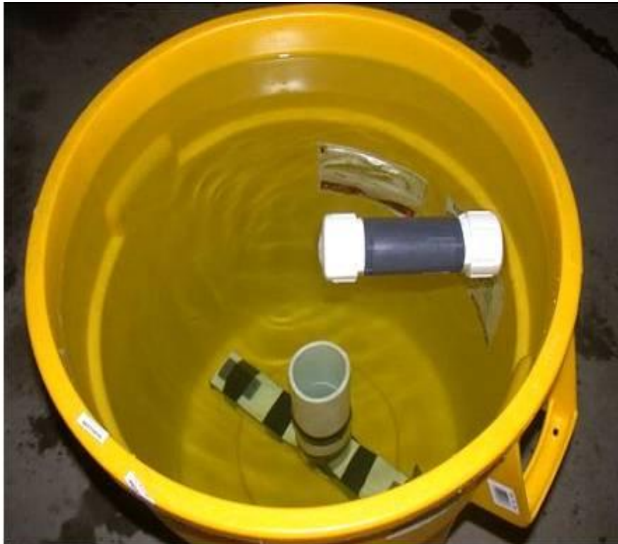
Figure 60: Rise Time Test After Sensor Release
