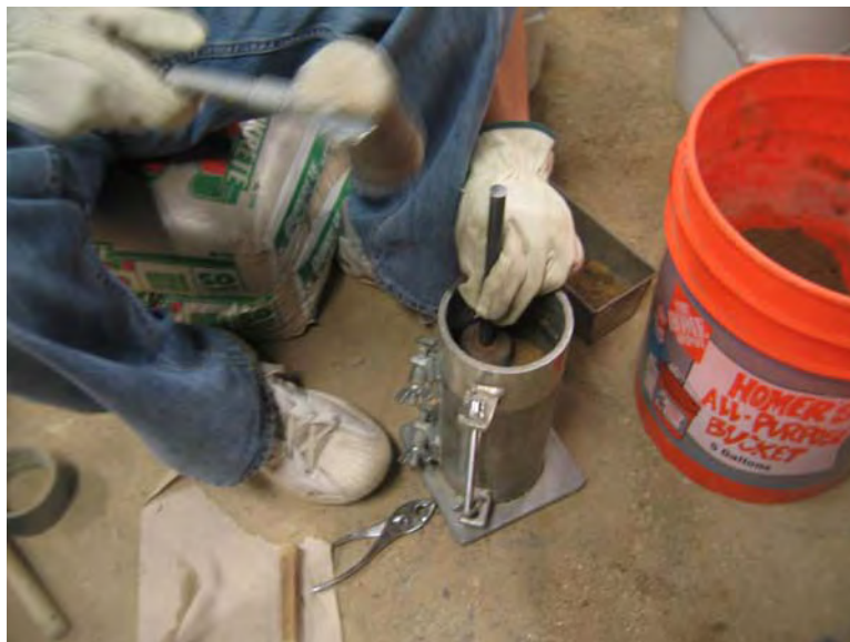
Figure 3-4. Preparation of 4.0 x 8.0 in. specimens
