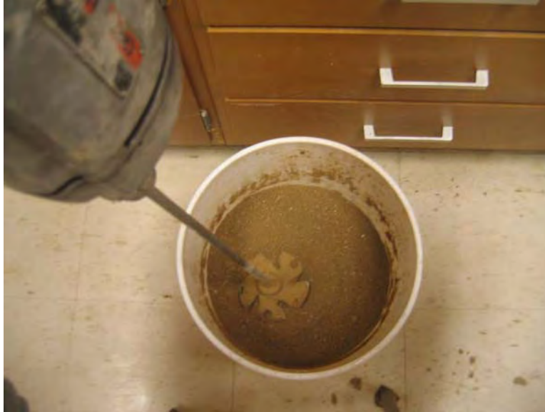
Figure 3-2. Laboratory mixing used for lime-treated soils 2 through 6
