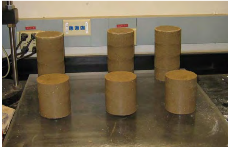
Figure 3-3. Two specimen geometries used during testing: 4.0 in. diameter × 4.5 in. tall and 4.0 in. diameter × 8.0 in. tall
