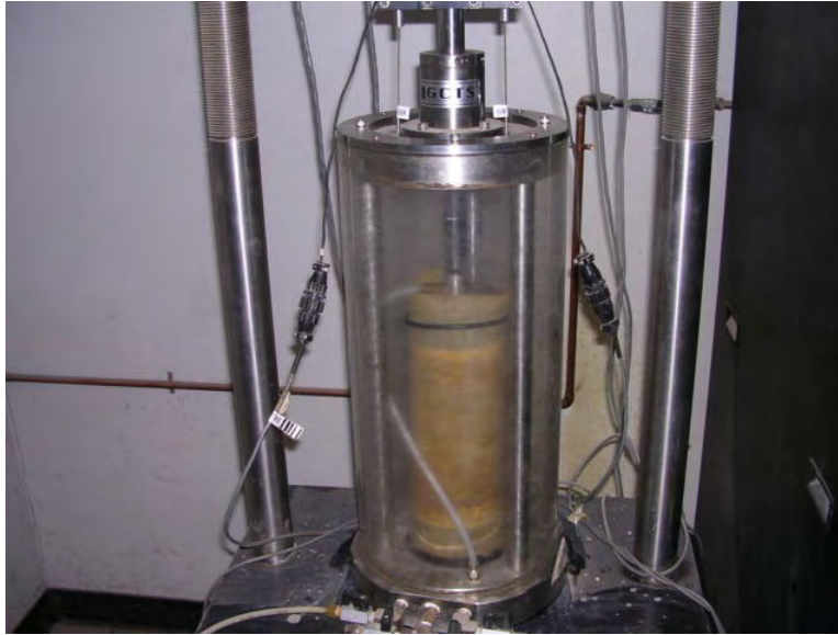
Figure 3-7. M_r test setup used by Ground Engineering
