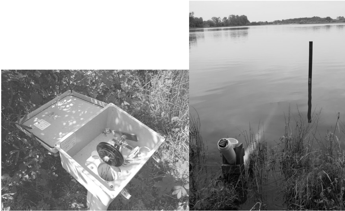
Figure 7. Image of pulley/float recording system showing the pulley, potentiometer, and the data logger on the left. Image of pit recorder and staff on right.
