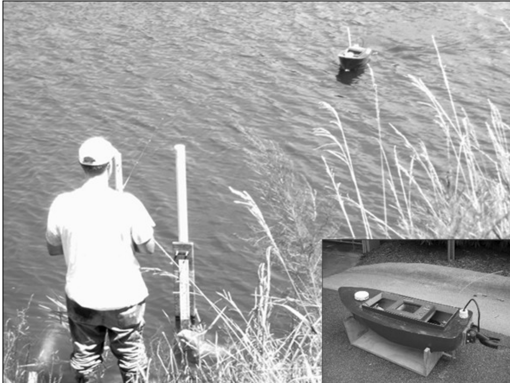
Figure 8. Sonar equipped model boat used to measure the depth to the restrictive layer in several study site borrow pits. Inset shows closer image of boat belonging to the Animal Waste Management extension program in BAE, NCSU
