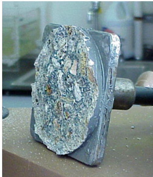
Figure C-3 – Showing panel/overpour bond is stronger than the overpour
