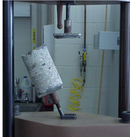
Figure C-2 – Core after failure in overpour
