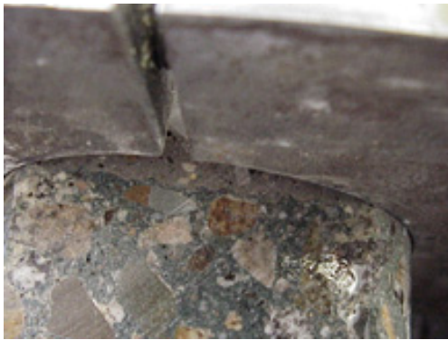
Figure A-4 - Lining up interface in device
