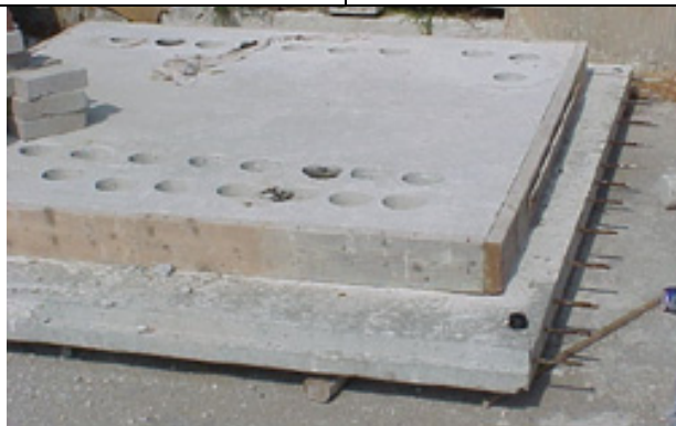
Figure D-3 – Control Slab with core holes
