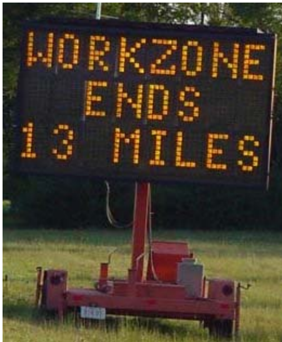
Figure 42. Changeable message signs informing drivers about the work zone (from [22]).
