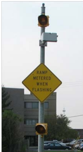
Figure 41. Advance warning sign for ramp metering (from [18]).
