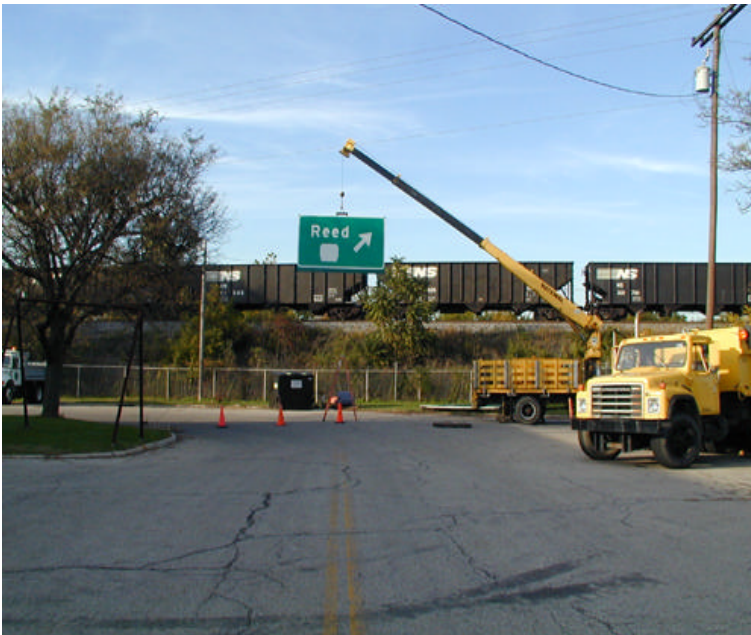
Figure 11. Experimental sign held at a height of 17 ft (5.1 m) by a crane in the ODOT sign shop parking lot. The sign was tethered to prevent movement.
