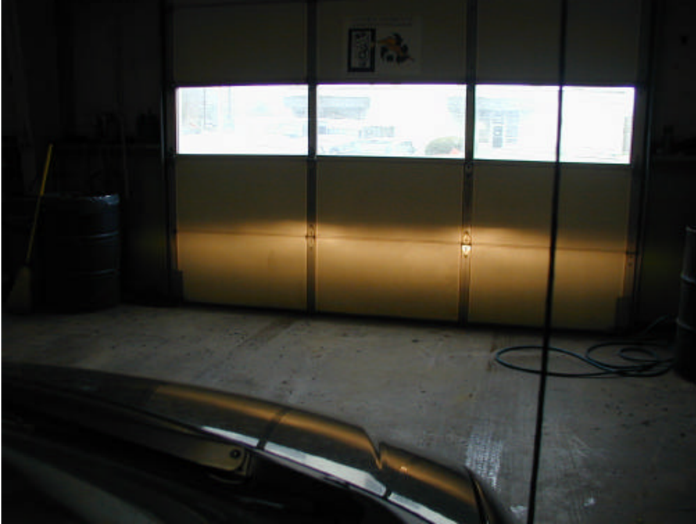
Figure 5. 2002 Dodge Caravan low beam headlamp pattern reflected on a garage door. Note the sharp vertical cutoff.
