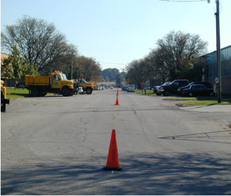
Figure 12. Traffic cones placed at 200 ft, 400 ft, 600 ft and 800 ft to aid in positioning the minivan for measurements.
