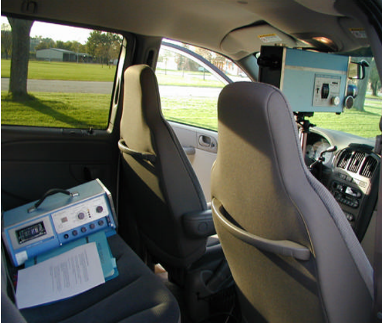
Figure 10. Pritchard photometer set up inside the 2002 Dodge Caravan. Measurements were actually made at night.
