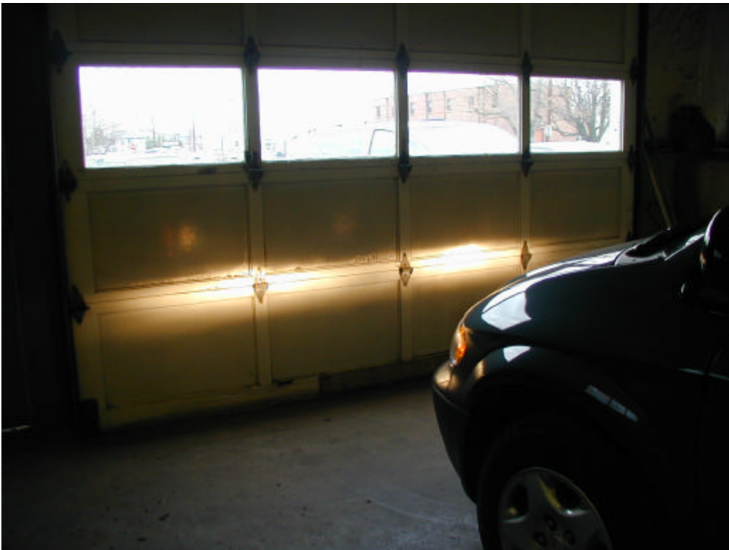
Figure 6. Close up view of Chrysler minivan headlamp pattern as seen in Figure 5, but with van closer to garage door.
