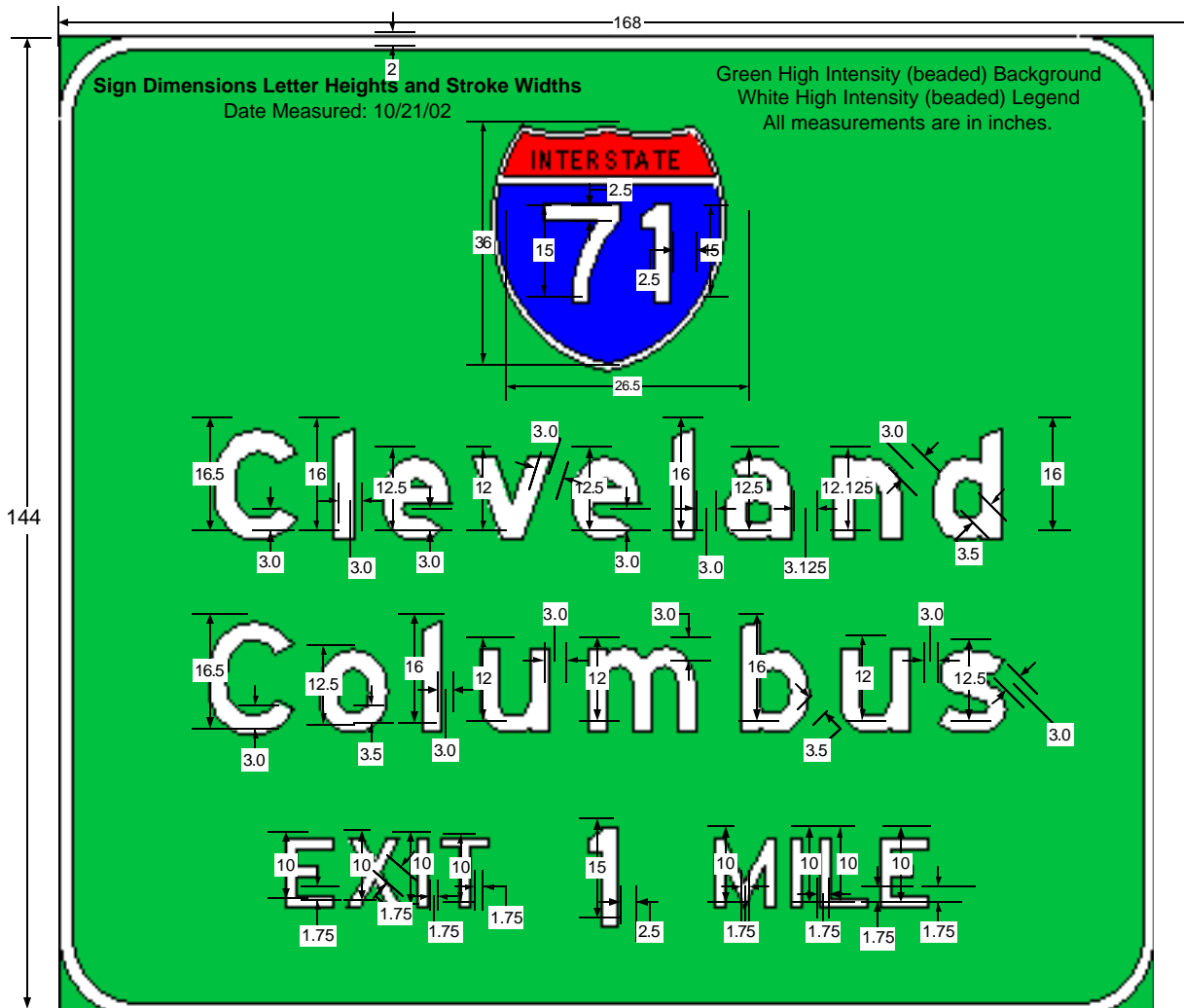
Sign Group C: Type VIII legend on microprismatic Type III background dimensions in inches. 1 inch = 2.54 cm.
