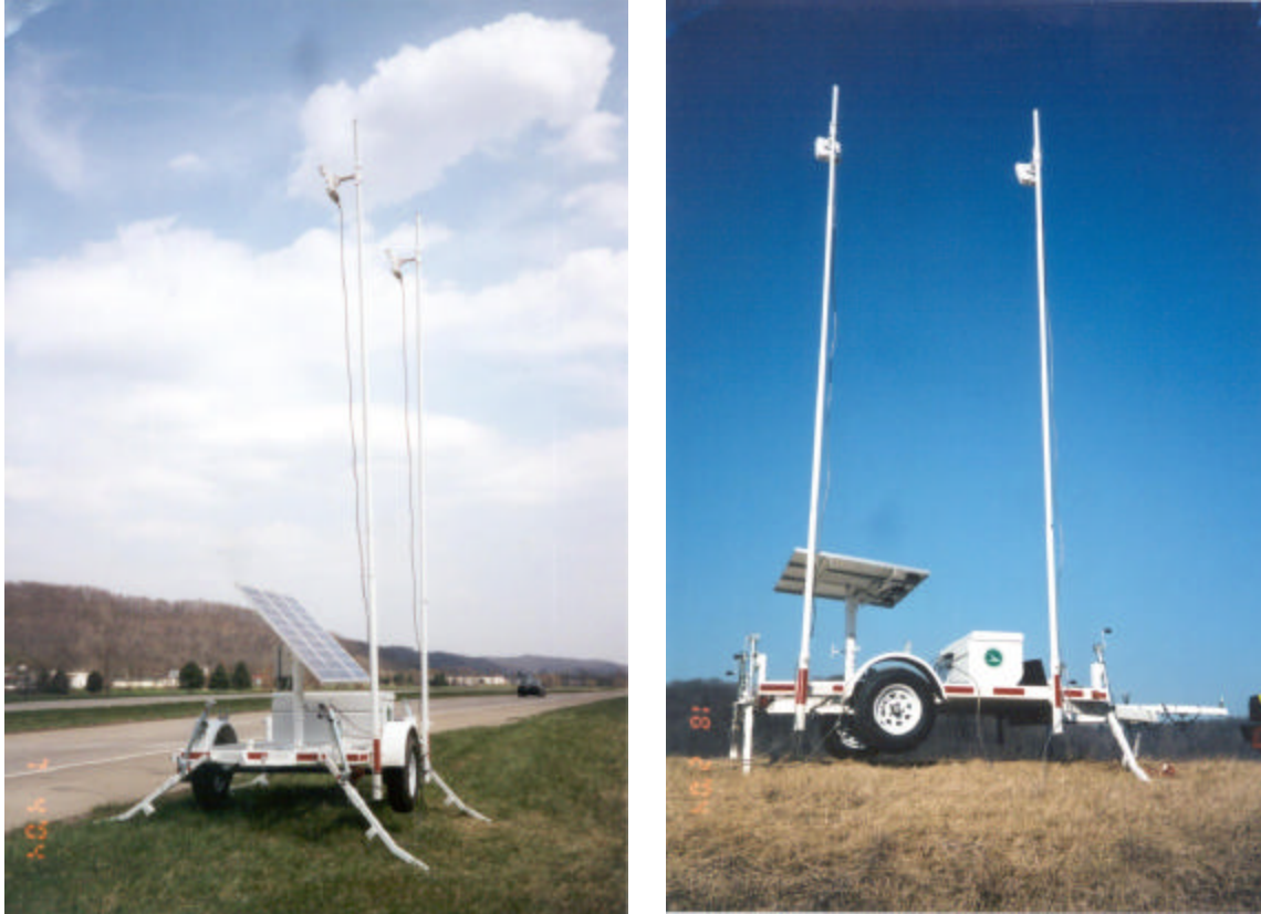
Figure 40: Microwave radar trailer set up to collect data a) rear view with solar panel in use, b) side view with solar panel in storage position
