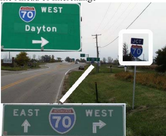
c. JCT 70, East West Guide Sign, and Cantilever Overhead Sign at First Gore
