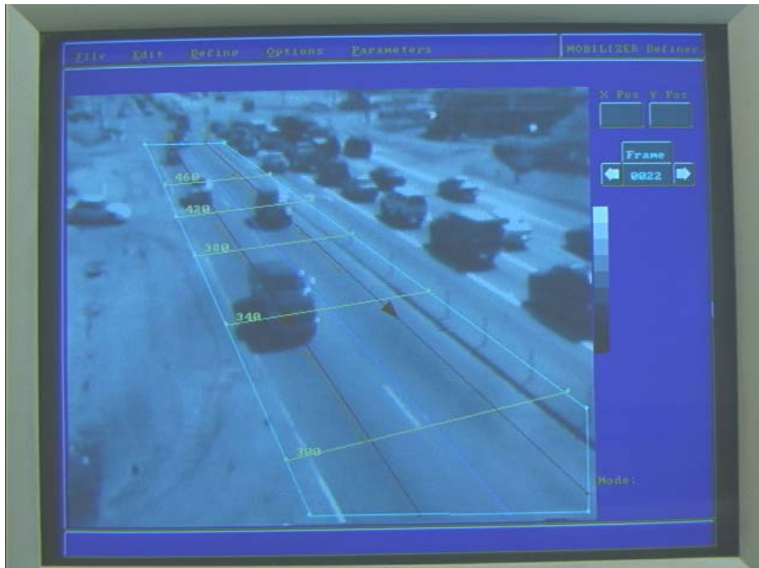
Figure 28. Mobilizer PC Geometry Definition at the First Camera Location, Brice Road
