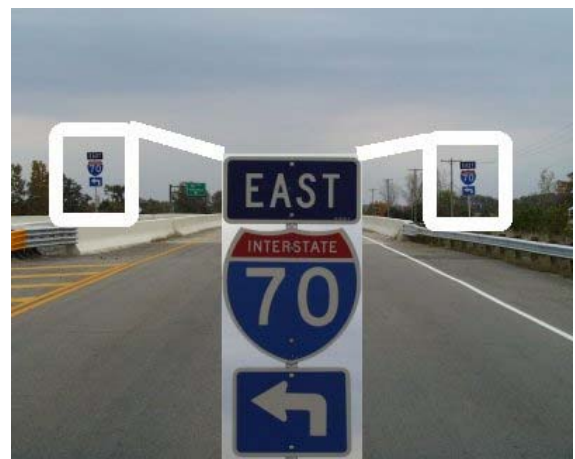
d. Trailblazer Assemblies on Bridge to Second Gore
