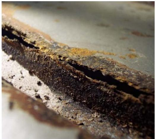
Figure 5-4b. Coupon #1 inside rib before cleaning.
