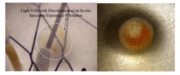
**Figure 7-6.** Light corrosion on a 2.54-cm (1-in) convex dimple immersed in solution P after 21 days of exposure (left) and severe corrosion on a 2.54-cm (1-in) convex dimple immersed in C solution after 19 days of exposure (right).
