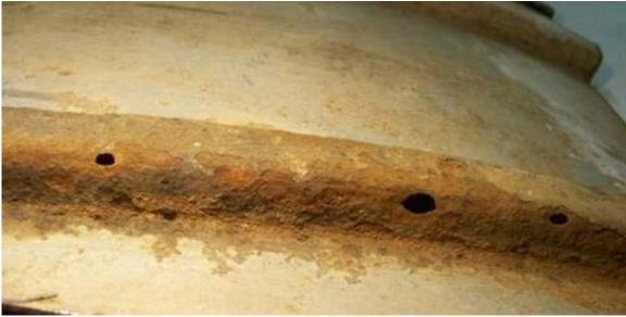
Figure 5-5. Coupon #4 outer rib after cleaning.
