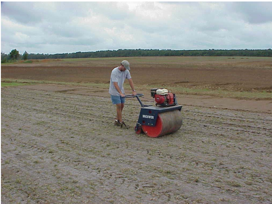
Figure 13. Areas established from sod, sprigs, or plugs should be rolled after planting.
