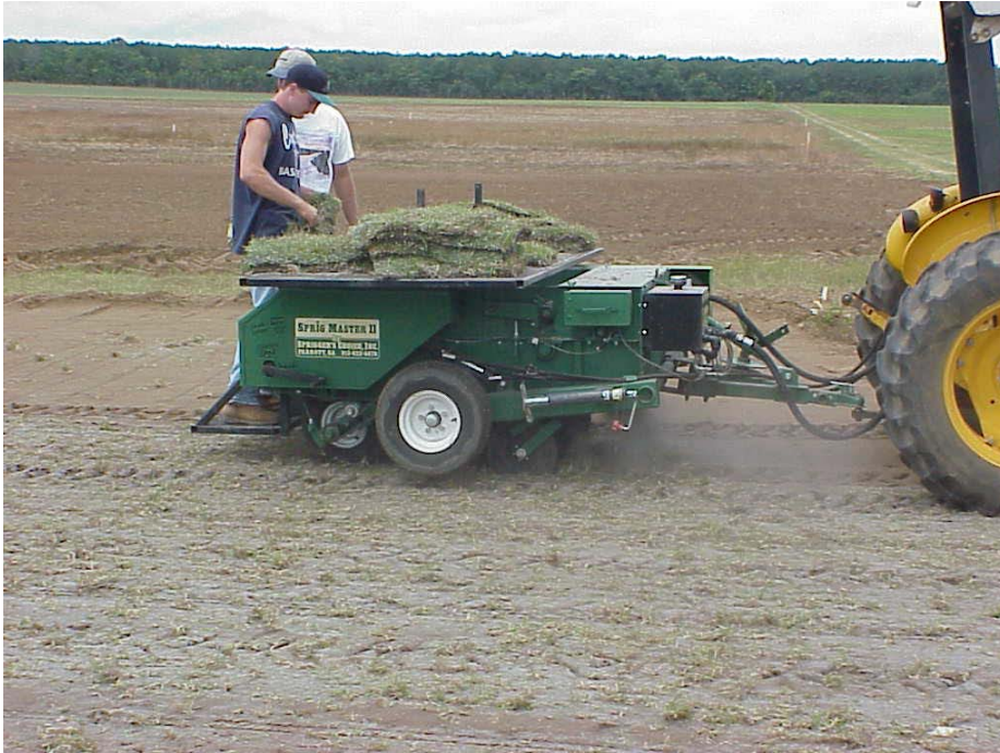
Figure 12. Sprigging of turfgrass using a sod-to-sprig machine.
