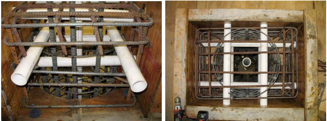
Figure 3.16 Formwork and PVC Layout on Loading Block
