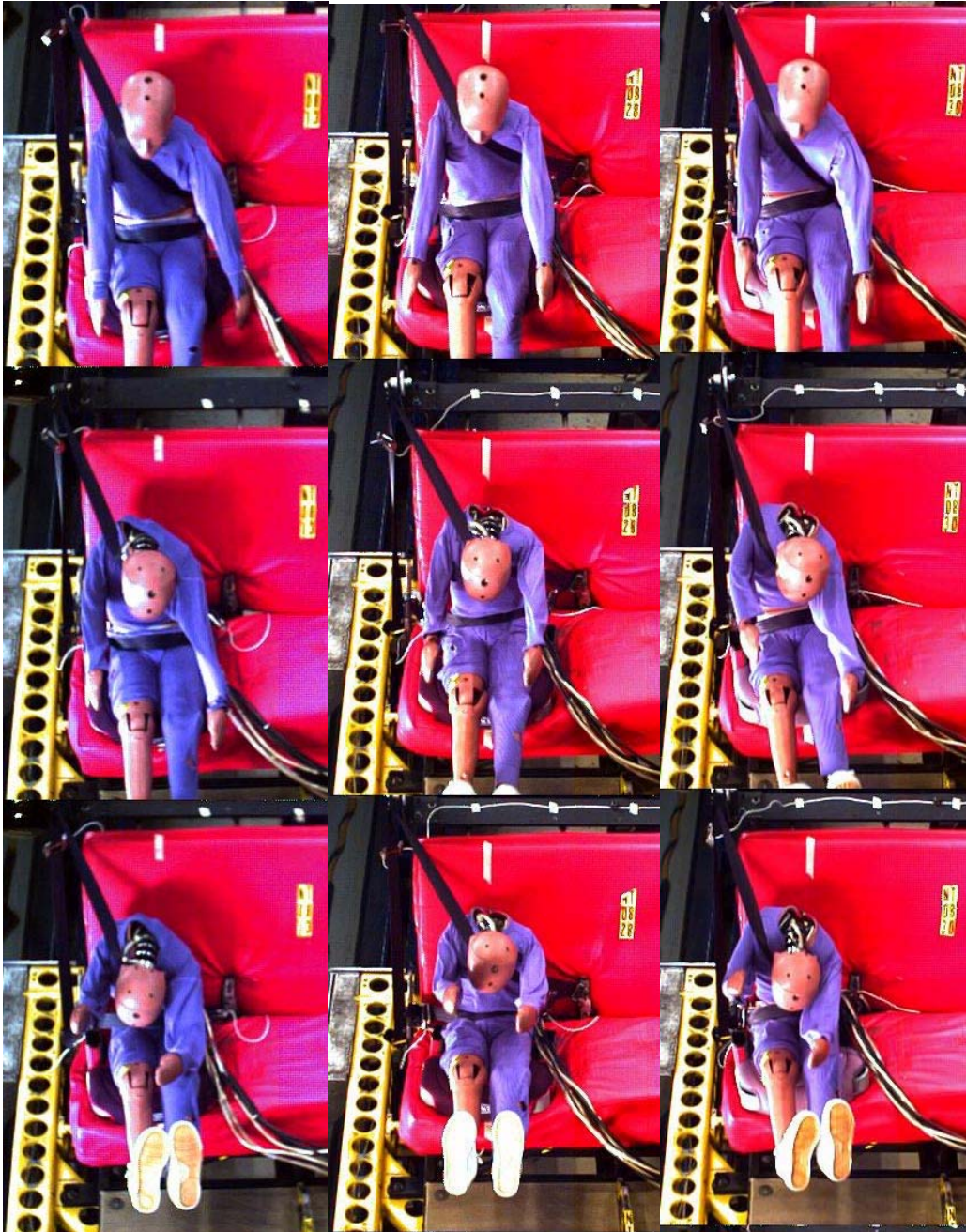
Figure 34. Kinematics with variation in lap belt spacing (from left: normal 213, 75 mm wider, 75 mm narrower). Frames from top to bottom are from times 80, 100, and 120 ms.
