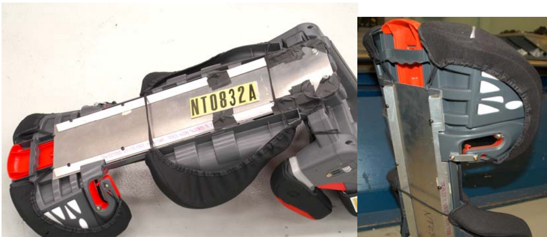
Figure 24. TurboBooster with structure modified to be more rigid, plus close-up of “closed” shoulder belt guide.
