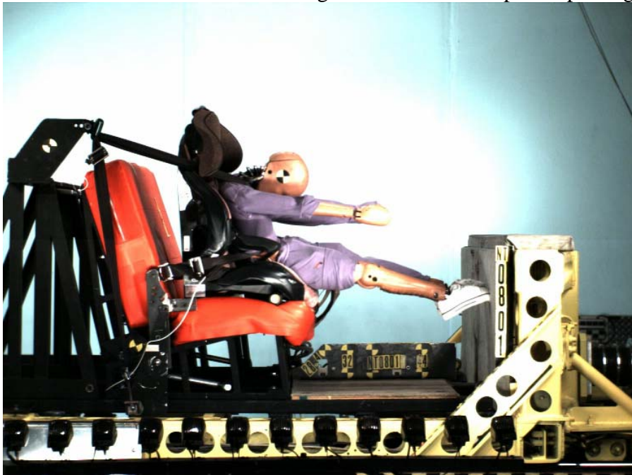
Figure 18. Peak excursion in test using Generations and poor lap belt geometry.
