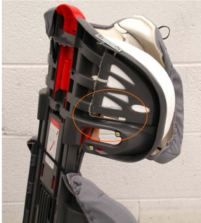
Figure 23. TurboBooster with modified slot design.
