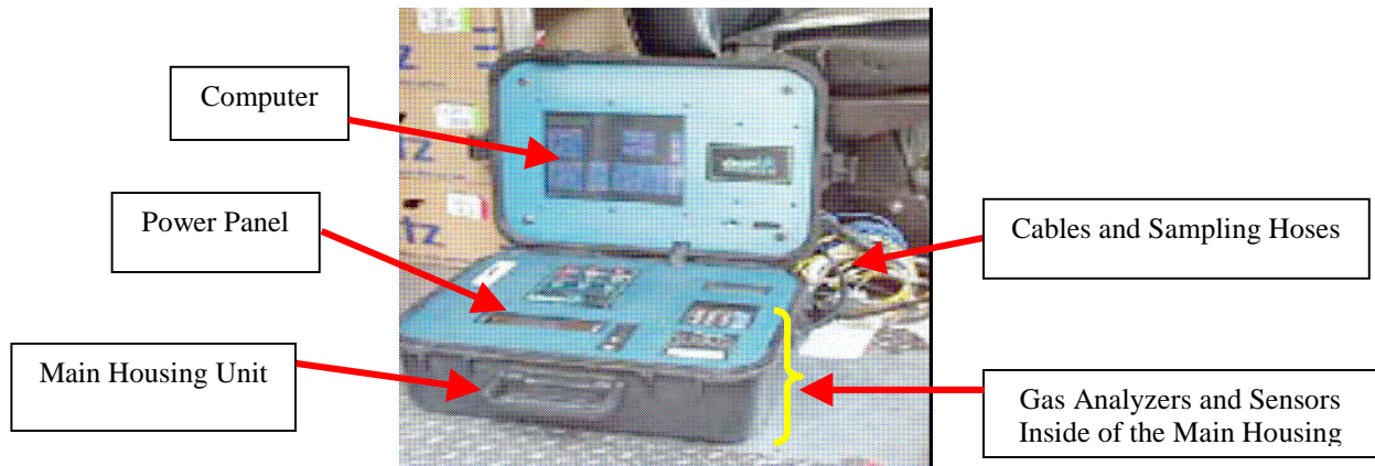
Figure 1. Montana System Components
