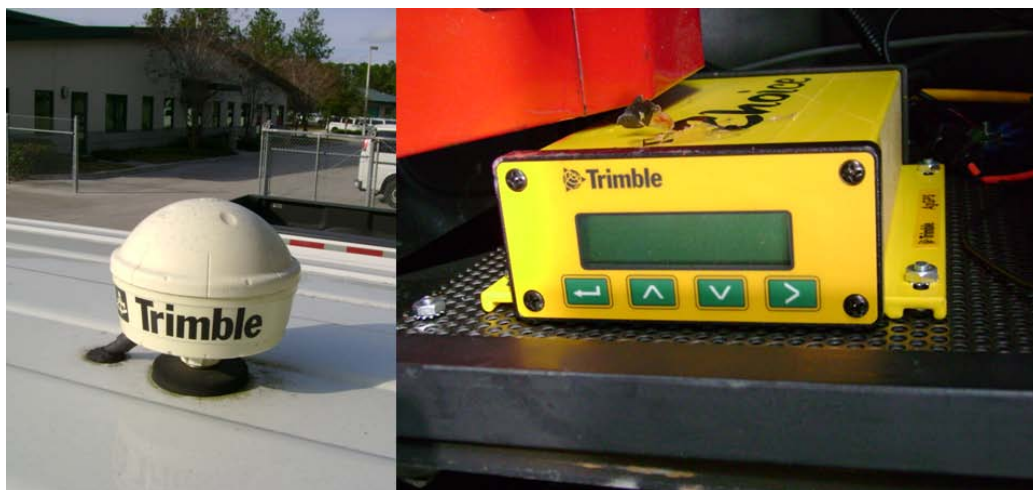
Figure 15. FDOT GPS Antenna and Receiver.
