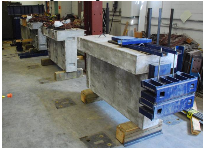
Figure 228: Disassembled beam for application of epoxy
