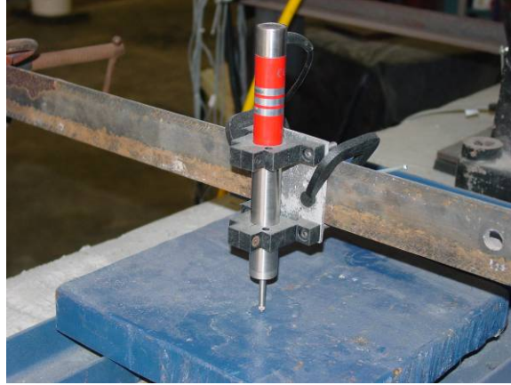
Figure 53 – LVDT for measuring deflection at cantilevered-end of beam
