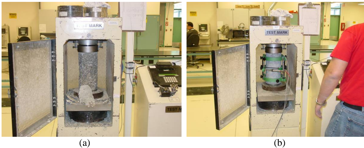
Figure 36 – (a) Compressive strength test setup; (b) Elastic modulus test setup
