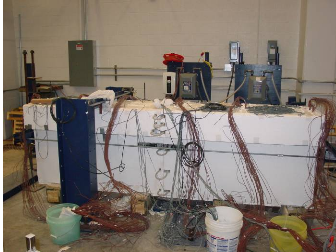
Figure 70 – Insulated heated segments
