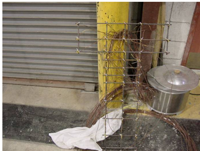
Figure 41 – Thermocouple cage with attached thermocouples
