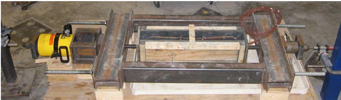
Figure 214: Load frame assembly prior to concrete placement
