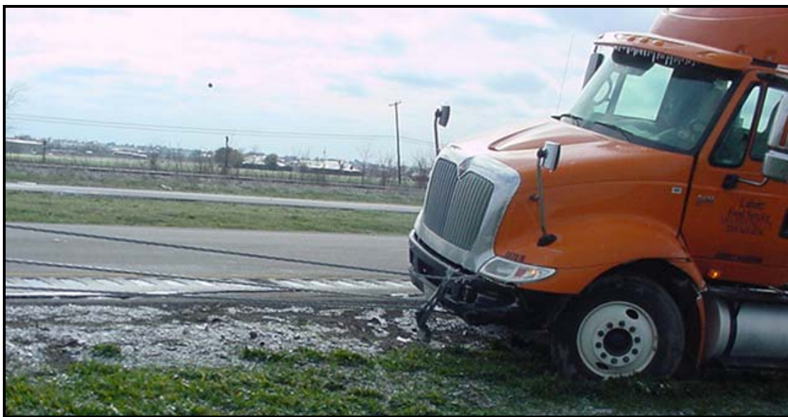
Figure 2-21. Successful Capture of Large Vehicle on I-20 in Kaufman County, TX.
