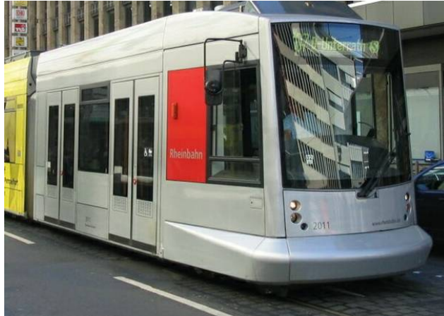
Figure 6. Low bumper profile on the Dusseldorf tram.
