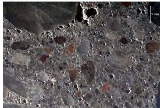
Magnification: 10x Description: Hardened air void system.
