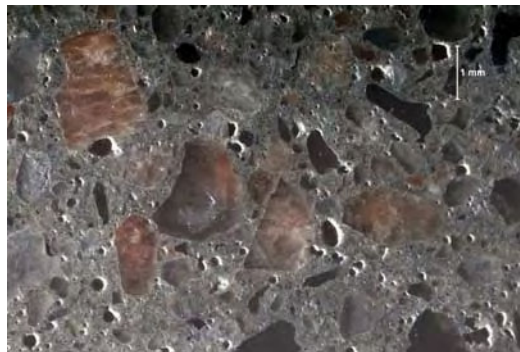
Magnification: 10x Description: Hardened air void system.
