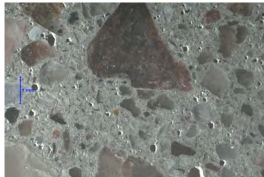
Magnification: 15x Description: Hardened air void system.
