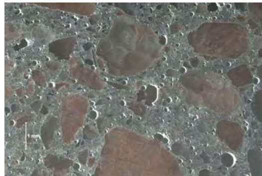
Magnification: 15x Description: Hardened air void system.
