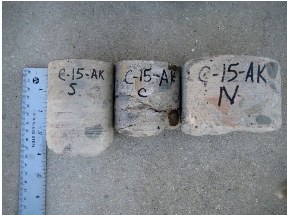
Figure 15. Core samples received by the laboratory for Structure C-15-AK
