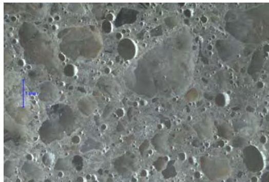
Magnification: 15x Description: Hardened air void system.
