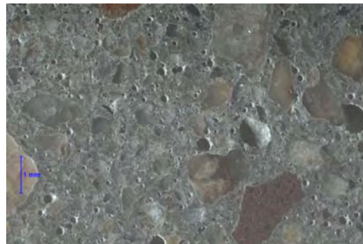
Magnification: 15x Description: Hardened air void system.
