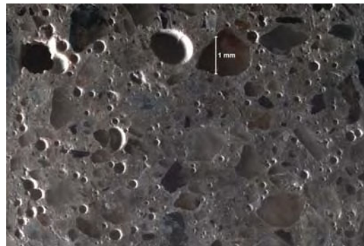
Magnification: 10x Description: Hardened air void system.
