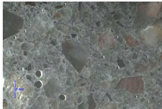
Magnification: 15x Description: Hardened air void system.
