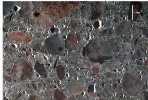
Magnification: 10x Description: Hardened air void system.
