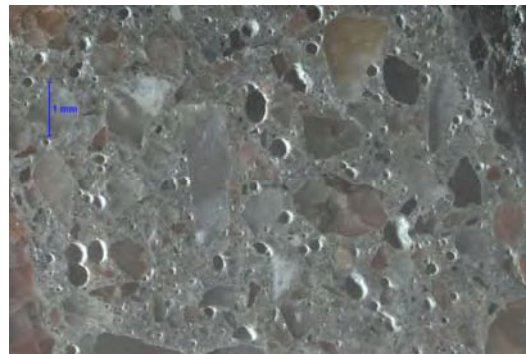
Magnification: 15x Description: Hardened air void system.
