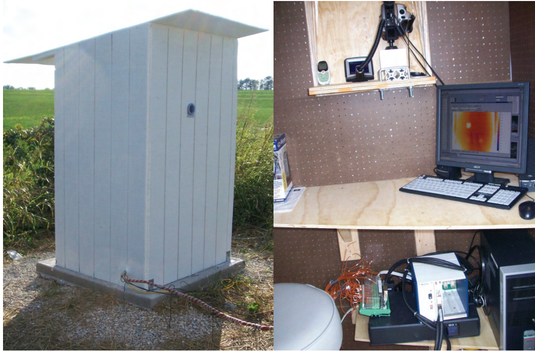
Figure 3.5 : Data house and inside layout with thermal imaging camera, standalone PC, and data acquisition (DAQ) equipment.
