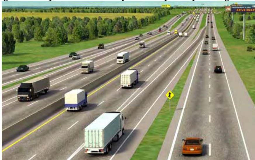
Figure 1 Proposed Truck-Only Lane Slip Ramp Configuration... 1
