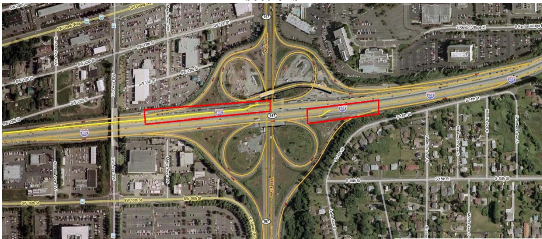
Figure 4-20 Two bottlenecks resulted from the enhanced capacities of upstream HOT lane sections
