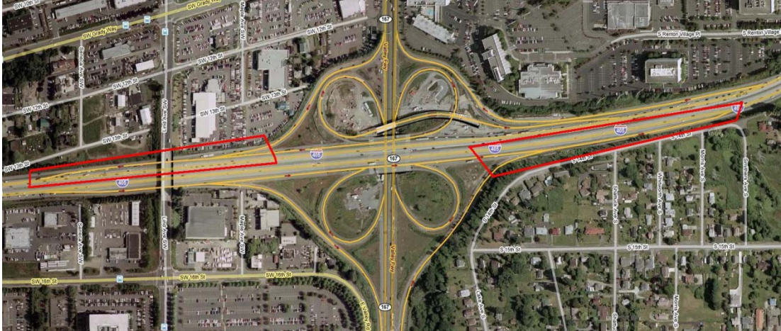
Figure 4-20 Two bottlenecks resulted from the enhanced capacities of upstream HOT lane sections
